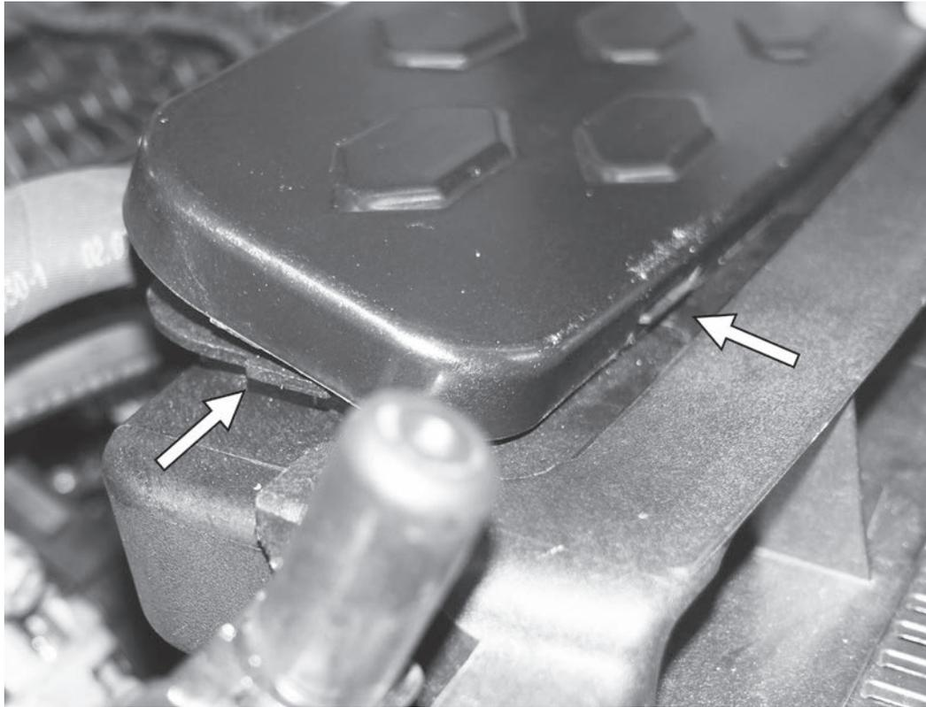
29) Install the airbox lid on the APR airbox by putting the front side of the cover on first. Ensure the two tabs on the front of the airbox go into the slots on the front of the airbox lid. Then, rotate the back of the airbox lid down. The lid will snap onto the tab on the right side of the APR airbox.
