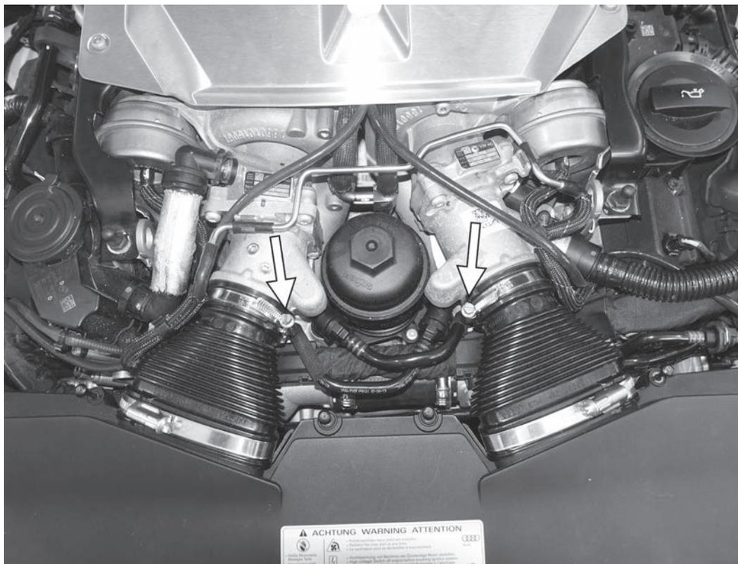
3) Loosen the two 7mm hose clamps holding the accordion hoses to the cast turbo inlets.
