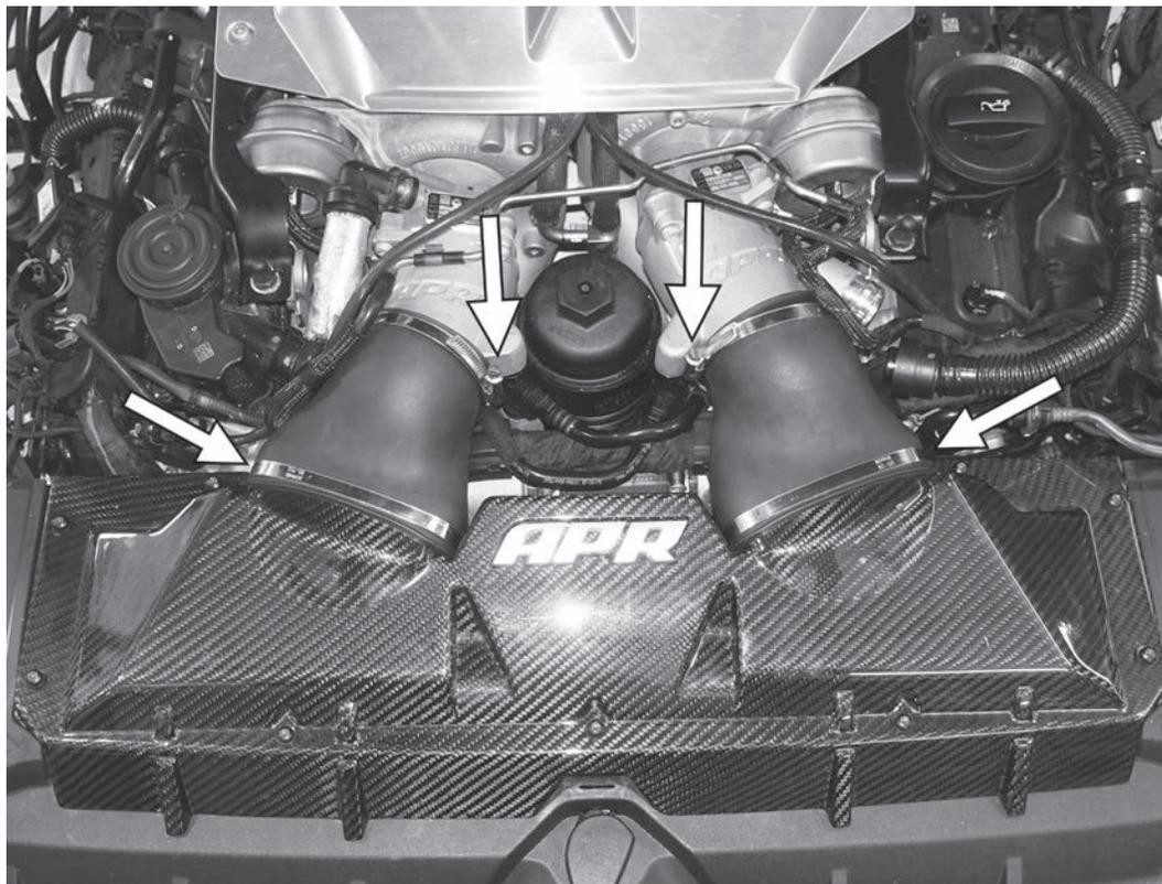
17) Adjust and tighten the clamps on the APR inlet hoses to the APR cast turbo inlet pipes, ensuring everything is seated unstressed. Torque all four 7mm screw clamps on both ends of the inlet hoses to 7Nm(62in-lbs).
