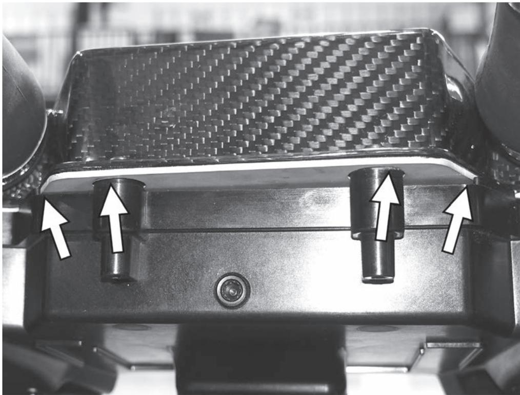
15) Tighten the two back screws between the APR inlet hoses first. Ensure the two plastic posts from the airbox base sit inside the metal plate of the APR airbox lid. As shown here, the post on the left side is seated inside the metal plate, the post on the right side is not. The posts have to be seated inside the holes on the metal plate, or the airbox will not sit down fully on the airbox base. Tighten the two T25 screws here to 1Nm (9in-lbs).
