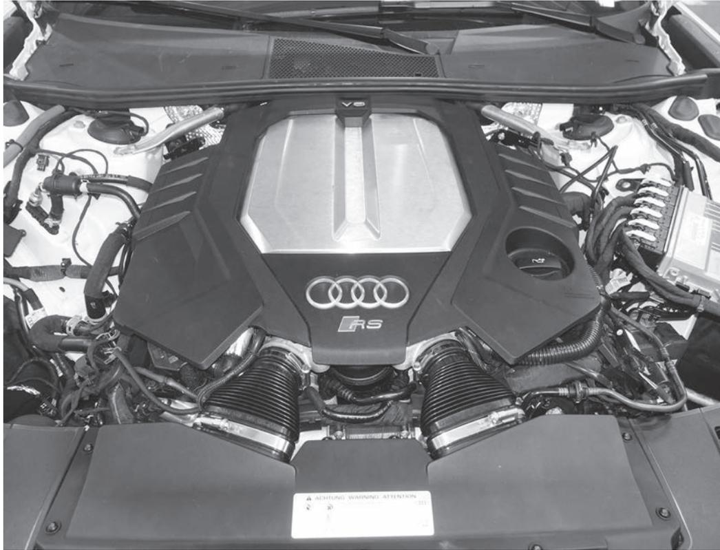
1) Raise the hood and remove the engine cover by lifting up on all four corners of the cover.
