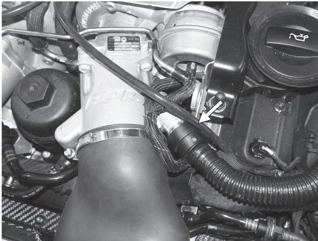
19) Reconnect the PCV valve to the right APR cast turbo inlet pipe by pressing it in place.
