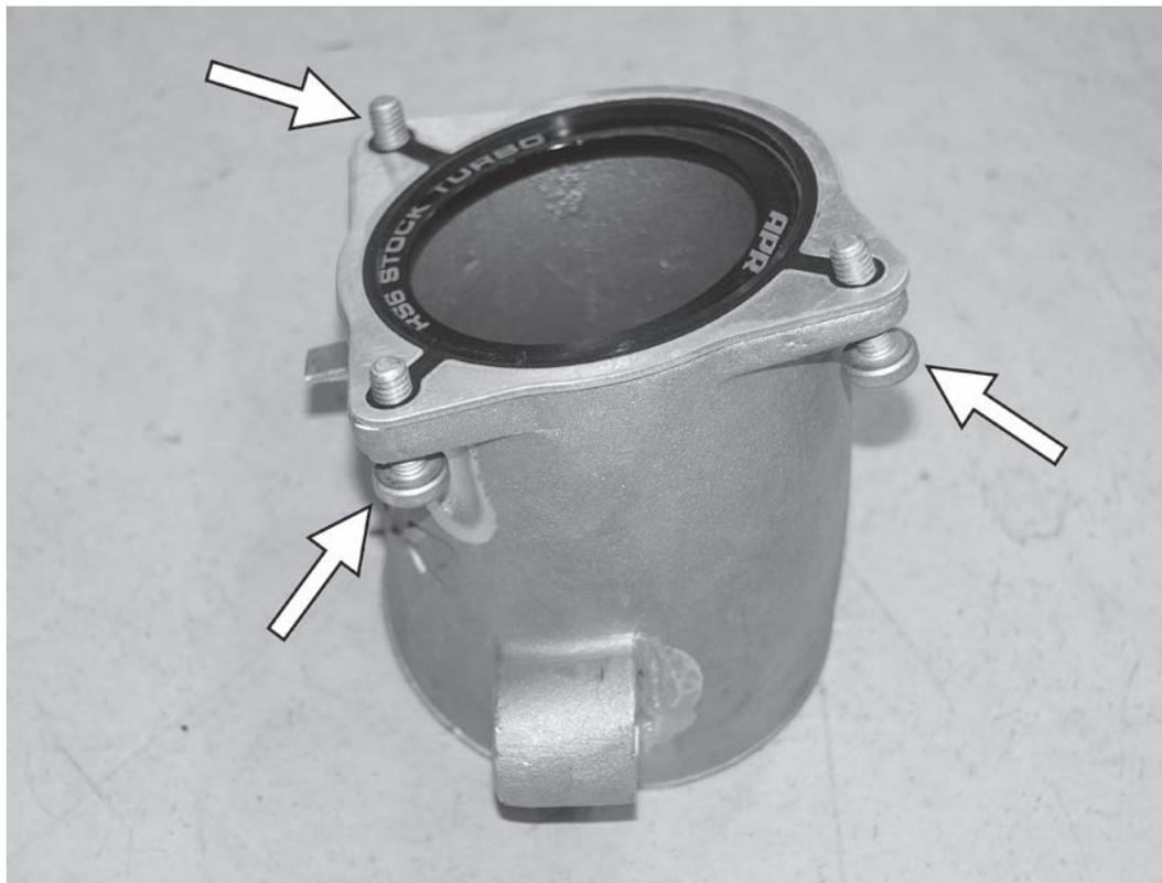
9) The inlet adapter ring for the stock turbos comes installed in the APR cast turbo inlet pipes. If using different turbos, uninstall the stock adapter rings and install the adapter ring for the turbos you are using. Place the supplied gasket on the inlet pipe flange, and loosely preinstall the six T30 screws through the casting and into the gasket. The gasket should retain the screws.
