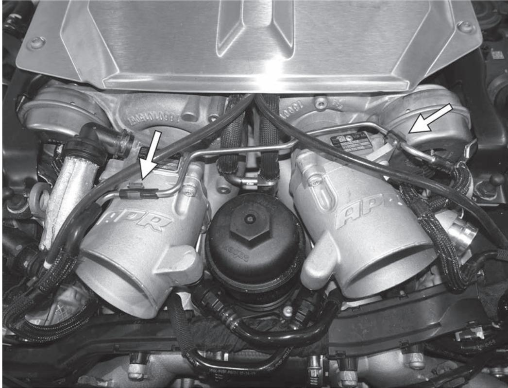
11) Reclip the hard vacuum lines onto the tabs on the top of the APR cast turbo inlet pipes.
