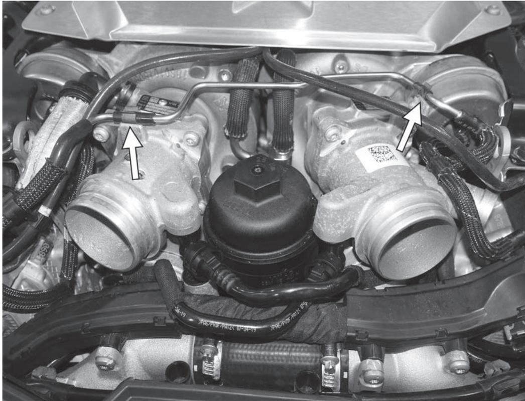
7) Unclip the hard vacuum lines from the top of the OEM cast turbo inlets.
