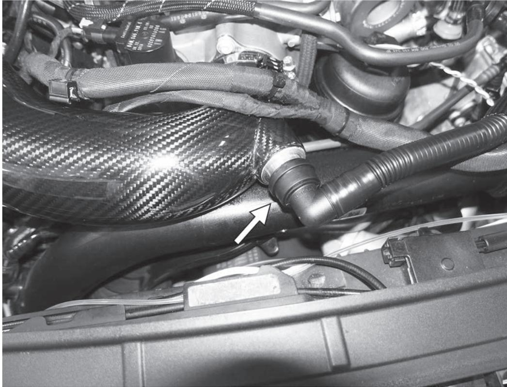
21) Reconnect the PCV hose to the front of the APR turbo inlet pipe by simply pressing the hose onto the port on the front of the inlet pipe.
