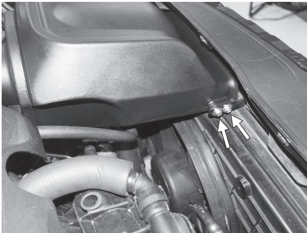
15) Using the supplied blue thread locker on the screws, install and tighten the two 3mm allen screws with washers to hold the front “L” bracket to the mounting bases on the front right of the APR intake.
