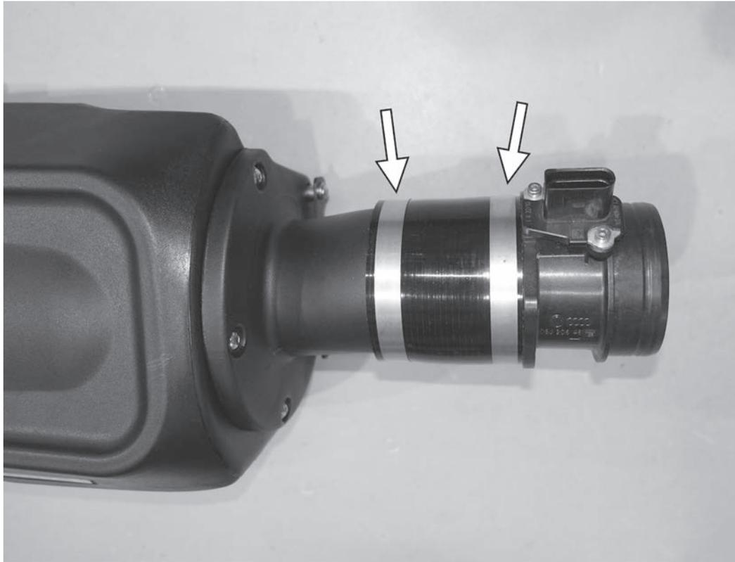
11) Using the supplied silicone coupler and two hose clamps, loosely install the MAF sensor to the back of the APR airbox in the same orientation as the with the stock sensor.
