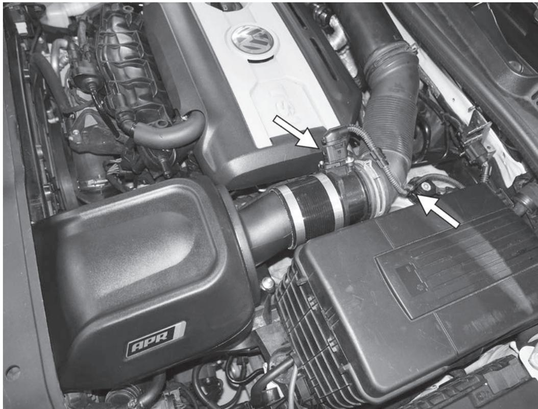
17) Reconnect the electrical connector to the MAF sensor. Reclip the MAF sensor wiring harness back onto the accordion inlet tube.
