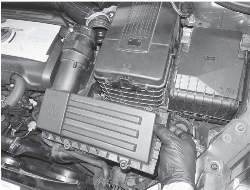
7) Lift the left side of the airbox up to pull off the rubber mounting post underneath. Lift the right side of the airbox from the other rubber mounting post to separate the airbox from the car.
