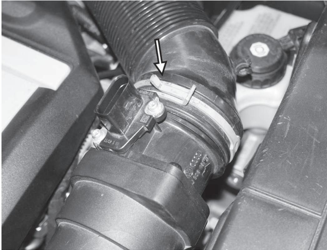
5) Squeeze the hose clamp holding the accordion inlet elbow to the back side of the MAF sensor, and slide the clamp off the MAF sensor. Separate the inlet elbow from the MAF sensor.
