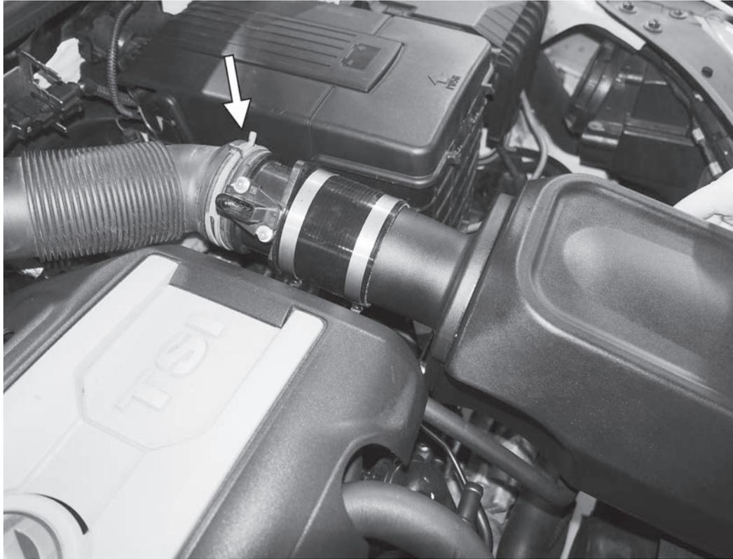
13) Loosely install the APR intake assembly in the car. Attach the according inlet elbow to the back of the MAF sensor housing and secure with the factory spring clamp.
