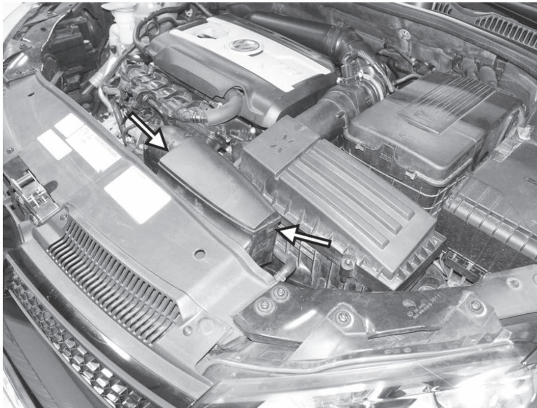
1) Lift up on the clips on both sides of the inlet scoop cover to remove the cover from the car.
