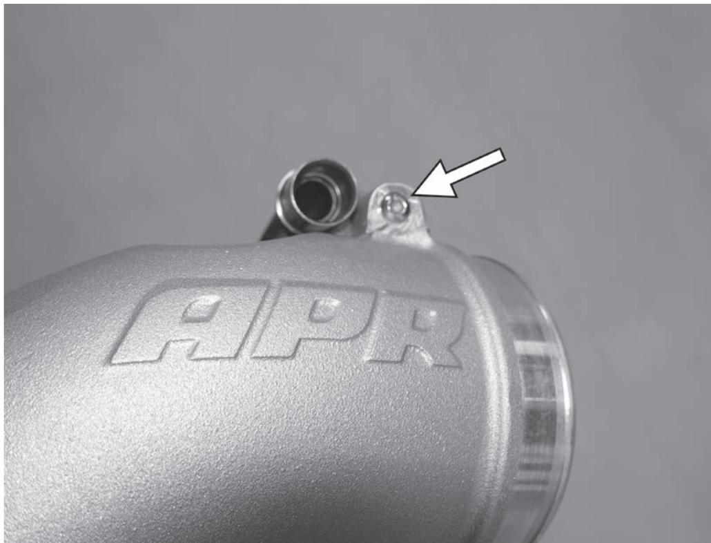
25) Remove the 4mm allen screw from the APR turbo inlet pipe and set aside for use later.
