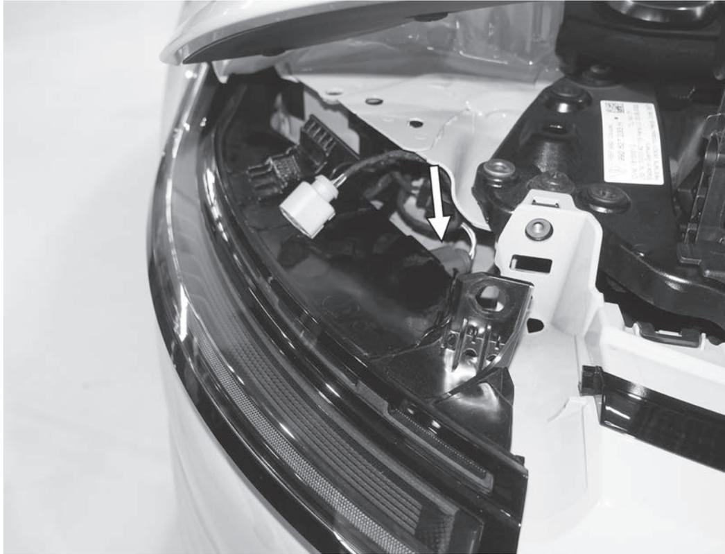
7) Pull both side taillight back slightly, and then disconnect the electrical connector from each light. Remove the lights from the car.
