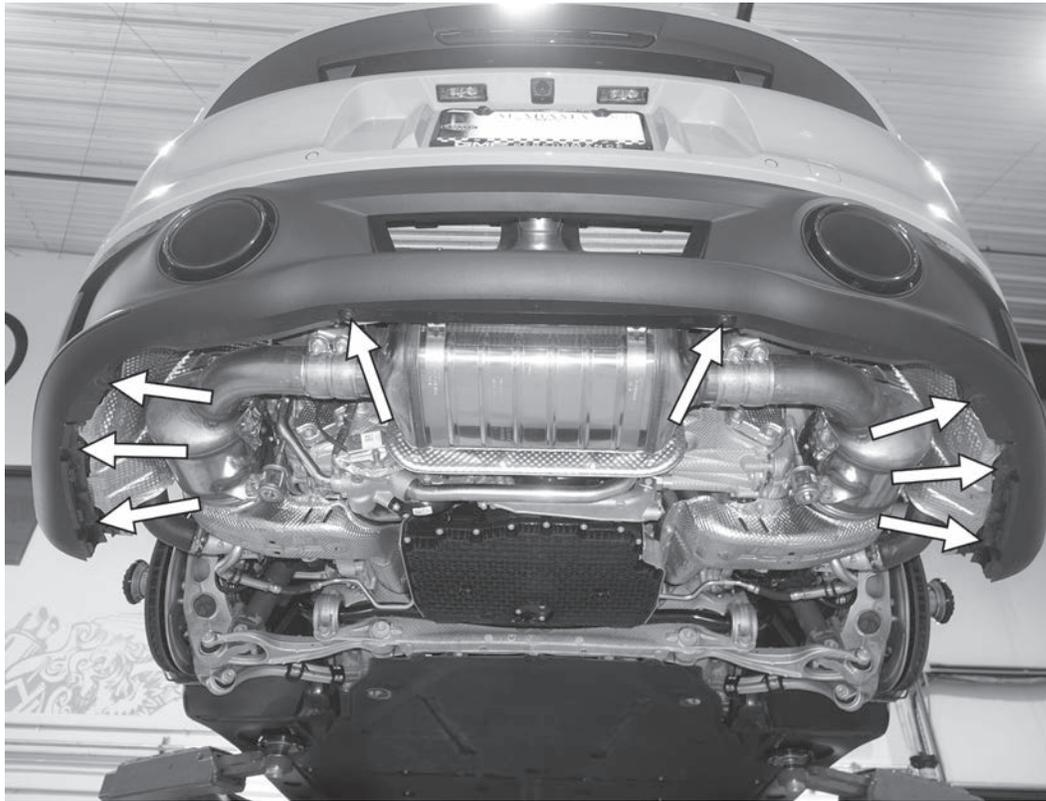
11) Remove the eight T30 screws from the bottom of the rear bumper. Note the placement of each screw and where it is located in the bumper.
