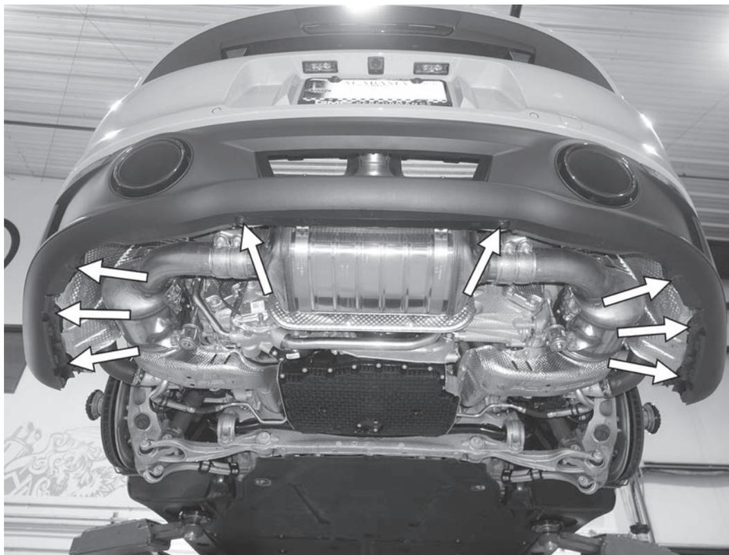
35) Reinstall the eight T30 screws from the bottom of the rear bumper. Make sure to put the correct screws in the same locations they were removed from. Tighten the screws to 3.2Nm (28 in-lbs).
