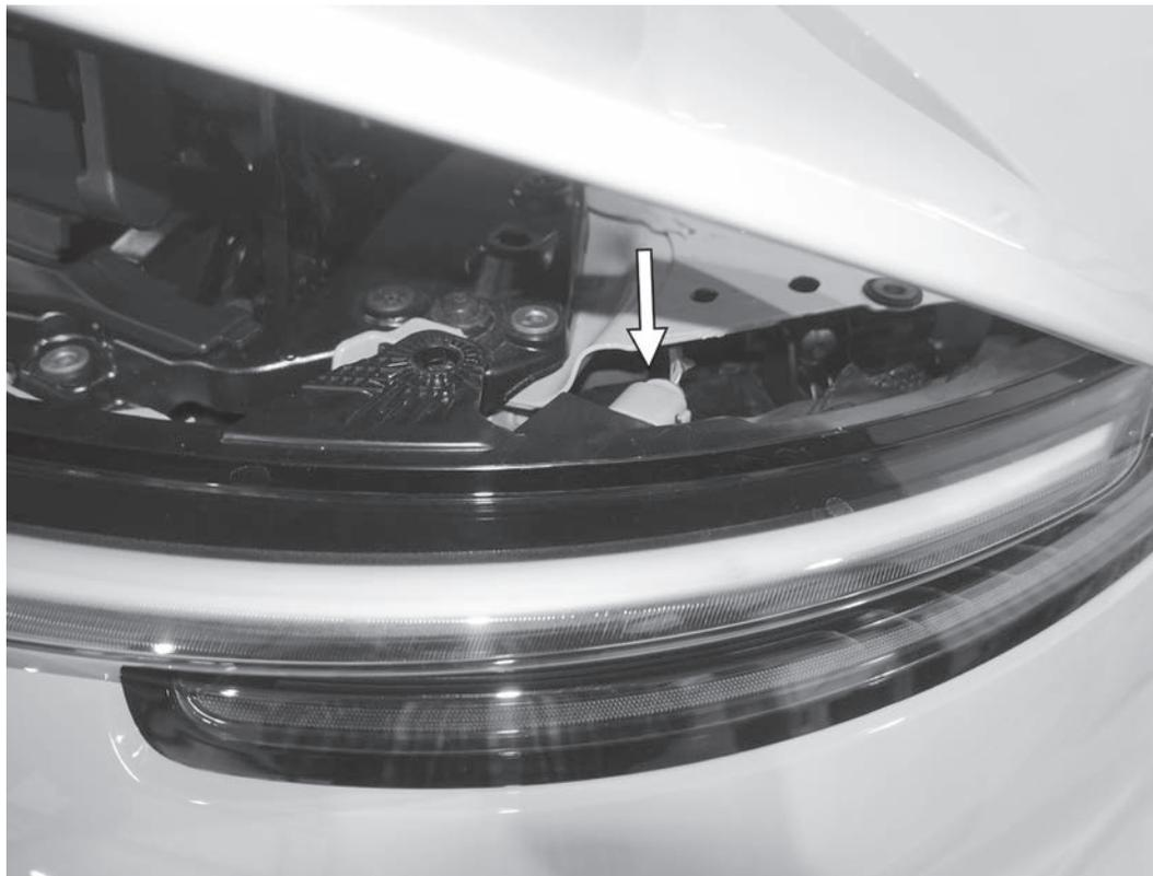
5) Pull the center taillight straight back a few inches from the car, exposing the electrical connectors. Disconnect both electrical connectors from either side of the center taillight and remove the taillight from the car.
