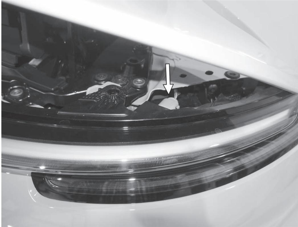
41) Place the center taillight back onto the car, and then reconnect the electrical connectors on both sides of the light. Push the taillight forward into its mounting location.
