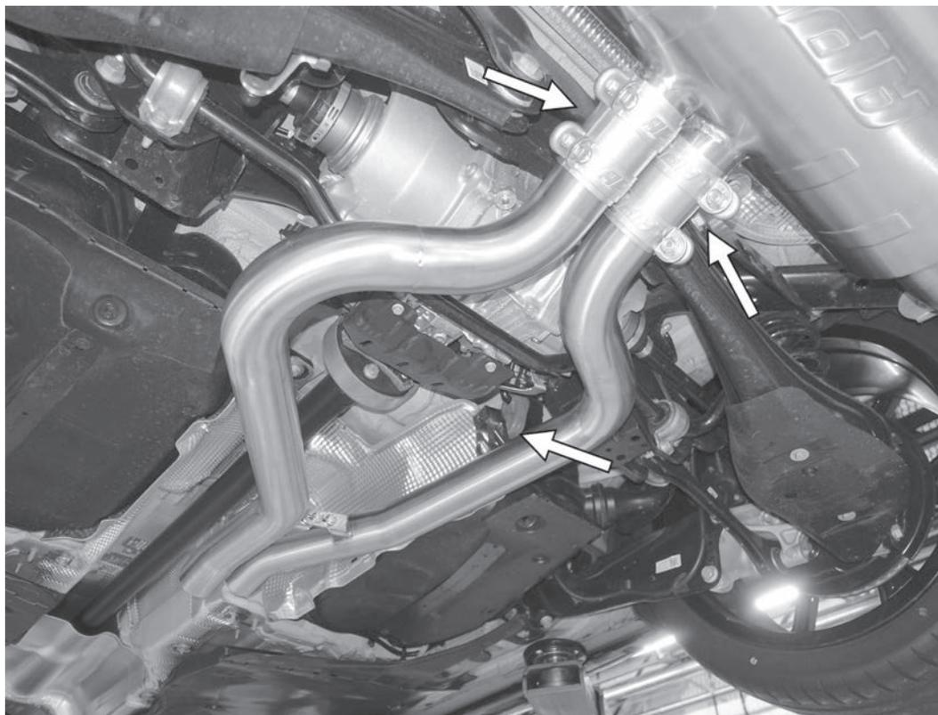
19) Loosely install the rear section assembly with two of the supplied APR sleeve clamps to the rear muffler as shown. Connect the exhaust mounting post onto the factory rubber hanger on the right side.
