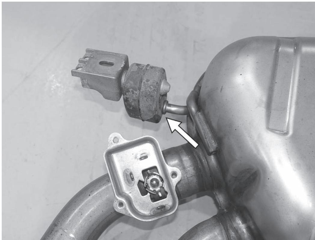
15) Remove the two exhaust hanger brackets with rubber mounts from the factory exhaust, and install them onto the APR exhaust in the same locations.
