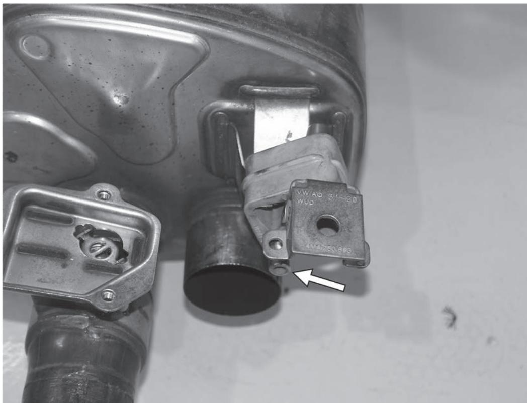
37) Remove both rubber exhaust hangers with their brackets from the factory exhaust, noting their orientation.
