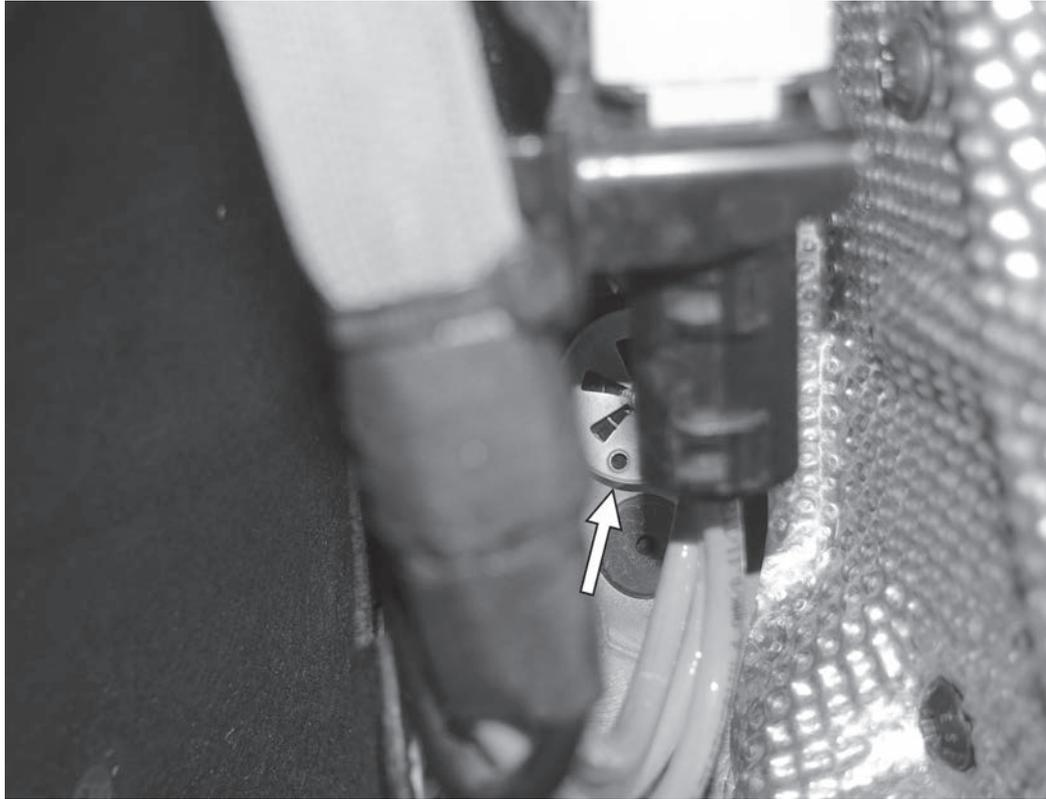
29) Reinstall the clamping washer on the back of the high voltage wiring harness bracket. The washer can be either spun into place, or pushed in place.
