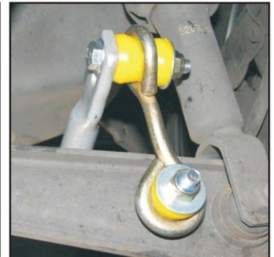
Photo 3. Link assembly - front view.
