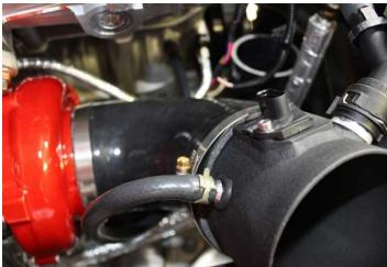
36. The smallest diameter hose will be used to replace the crankcase vent tube that routes from the engine block to the factory intake. Using the same engine block fitting, this hose will route to the barbed fitting on the powder coated intake pipe. Use the red spring clamp on the engine block side and the green clamp on the intake side.
