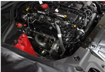
4. Push the white locking tab up and remove the electrical connector on the airbox. Then, using a flat blade screwdriver or 6mm socket, loosen the clamp holding the intake tube to the airbox. If your car is equipped with a strut tower brace, now would be the time to remove it.
