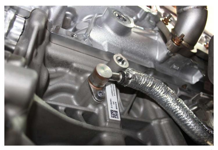
28. The oil return line will route through the motor mount to the -8 AN fitting in the block. Use a dab of silicone lubricant on the threads to prevent them from galling.
