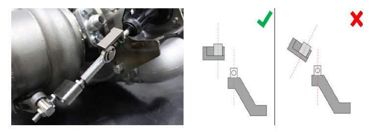
25. With the wastegate linkage all set up, you can clamp the turbo to the manifold and get it installed on the engine. Orient the v-band clamp as shown for easy access once the turbo is installed.
