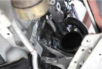
12. With the downpipe out of the way you can start removing the oil and coolant lines from the engine block. All of these lines are held in place with T27 Torx head bolts. Start with the rear coolant return line. There will likely still be coolant trapped behind this fitting so it is a good idea to have a drain in place and some shop rags handy. Remove the bolt on the fitting itself as well as the rubber support clamp bolt. Once both bolts are removed, grab and wiggle the fitting out.
