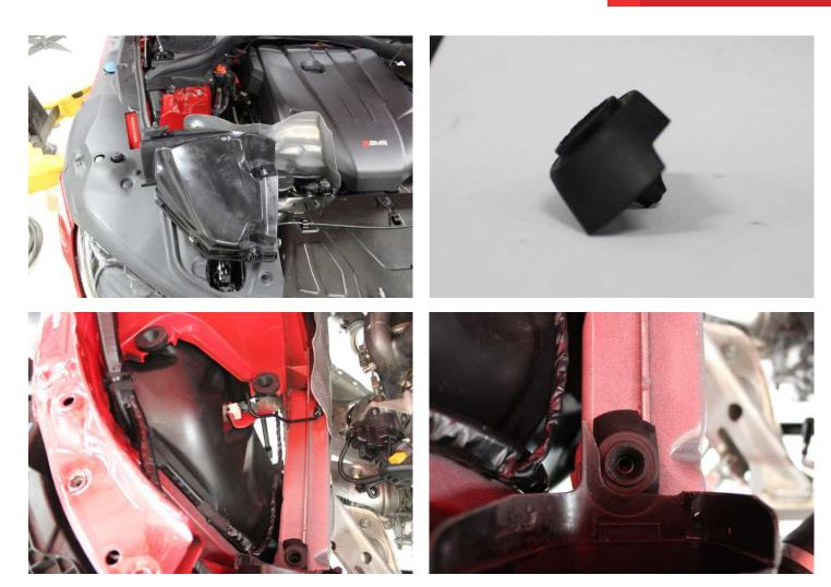
8. Remove the intake tube. First release the "C" shaped retainer clip holding the tube to the compressor inlet as shown. One end is visible on the top, the other end is underneath the tube.
