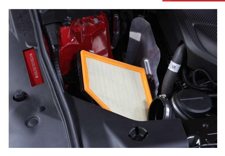
7. If the grommets came out with the airbox, remove them from the air box and reinstall them back in the car.
