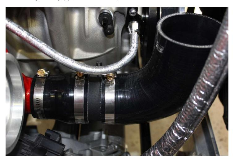
32. Install the adapter onto the throttle body and transfer the sensors to the new charge pipe.
