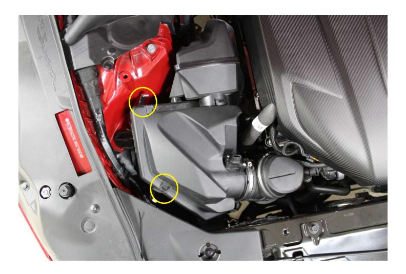
6. There are three grommets holding the air box in. One on the side and two underneath. Grab ahold of the lower airbox assembly and pull it straight up out of the grommets one at a time.
