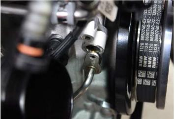
14. The oil drain fitting is located directly under the turbo. Remove the bolt and wiggle the fitting free.
