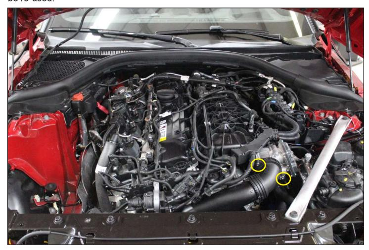
10. With everything disconnected, you can now remove the factory charge pipe from the engine bay. To make this easier, you can remove the bracket that mounts the small electric water pump to the front of the engine. Leave all hoses connected and remove the 10mm nut on the bottom of the bracket. This will provide you more space to pull the charge pipe out without damaging anything.
