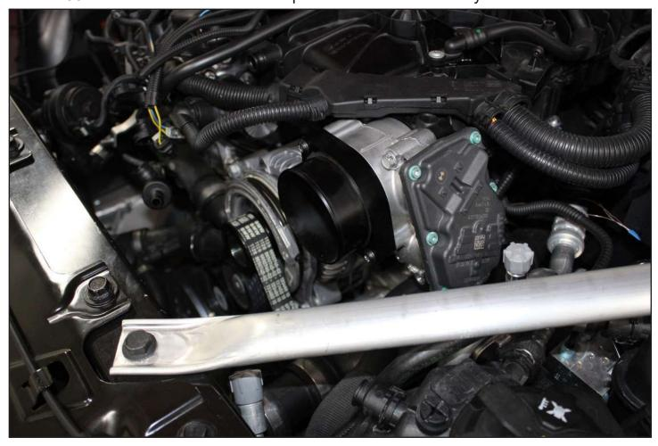
12. Remove the spring clip from the turbo side of the factory charge pipe and install it on the compressor adapter. Push the adapter onto the turbo and ensure that the spring clip sits in the slot on the compressor outlet.
