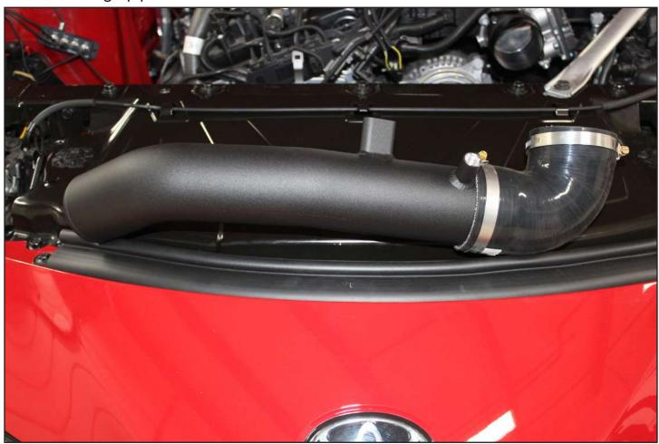
15. Transfer the two sensors from the stock charge pipe to the new one.
