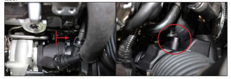
7. Unplug the two sensors on the charge pipe near the throttle body. Pull the white tabs out and press down while pulling on the connectors to remove them.
