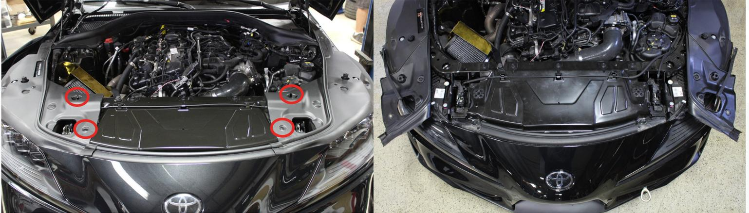
2. Remove the front hood seal and the six 10mm bolts underneath. Gently pull the nose piece of the bumper free of its mounting clips. With that out of the way, you can gain access to the 13mm cover panel bolts. Loosen the four front bolts and remove the rest. Unclip the hood release cable and the panel will slide backwards and then pull up.
