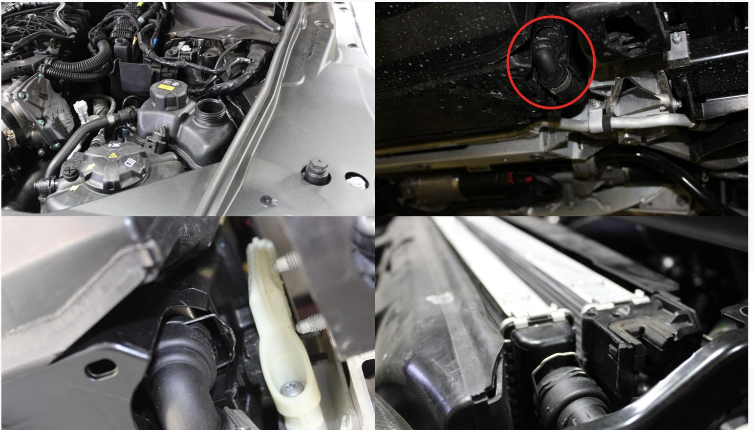
5. With the factory heat exchanger removed, the mounting brackets for the transmission cooler will need to be slightly modified to account for the extra width of the AMS heat exchanger. There are a few different ways to do this, explained in the following steps.
