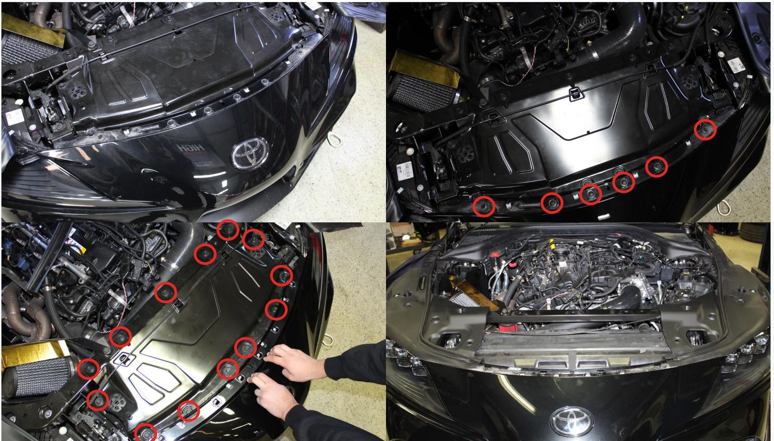
3. Next, remove the two T30 screws holding the plastic radiator cover in place. It is clipped into the fan shroud and will need to be unclipped to remove. If the cover is difficult to remove, try lifting up on the fan shroud slightly to create more clearance for the cover.
