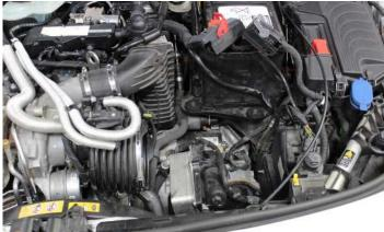
**6)** Drain the intercooler system. The lowest point in the system is the lower water hose connector on the side heat exchanger on the right side of the vehicle. Remove the fender liner and drain the system from there. The system can also be drained from the bottom connection on the intercooler or the intercooler pump however it will be a little messier.
