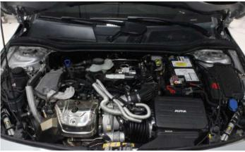
**2)** Once the battery covers and cables are removed, go ahead and remove the battery hold down brackets and plastic enclosure. Once that is done, remove the battery from the vehicle.
