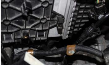
**10)** Disconnect the small quick connect line going into the top of the intercooler outlet end tank as well as the MAP sensor harness on the side.
