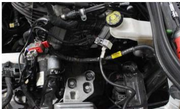
**8)** Loosen the hose clamps on the factory intercooler inlet coupler and outlet coupler. New hose clamps have also been provided for these connections with the new intercooler.
