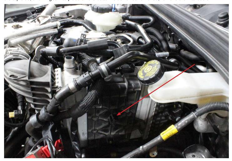
**13)** Remove the factory MAP sensor that is fastened to the OEM intercooler and install it onto the flange on the Alpha Intercooler using the supplied hardware. Make sure NOT to reuse the OEM bolts as damage will occur to the new intercooler.
