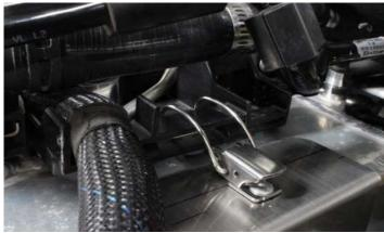
Note: Replace the OEM clamps on the compressor discharge and intercooler outlet coupler with the two #40 and one #56 clamp provided. Make sure to tighten the clamp as close to the bead on the inlet and outlet to deter movement.
