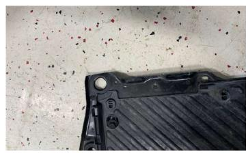
**17)** The air box mounting bracket may also need trimming. Test fit the air box and trim the mounting bracket as necessary to clear the intercooler end tank.
