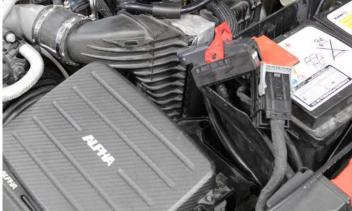
**4)** Disconnect the MAP sensor on the air box. To do so, use a small screwdriver to pull out the grey tab from the connector. Once released, depress the grey tab down to disconnect.
