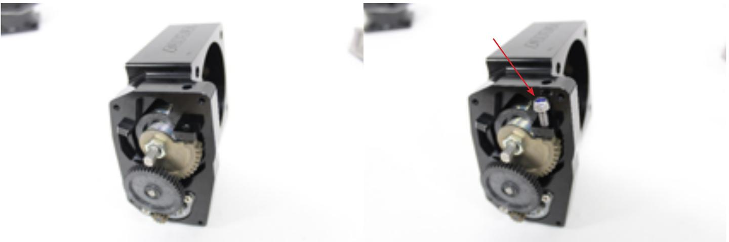
20. When closing the throttle plate by hand, you may notice that it “sticks” closed. To set the adjustment of this set screw, you will thread it in clockwise just until you can close the throttle by hand without it sticking. You want the throttle plate to seal as much as possible without it sticking closed. Once a position has been determined, hold the adjustment of the screw steady and then tighten the locking nut.
