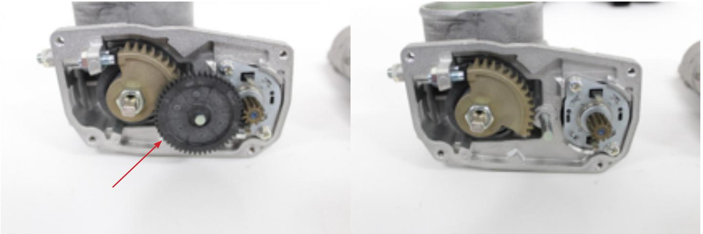
6. Remove the two screws securing the Drive motor. Remove the motor.
