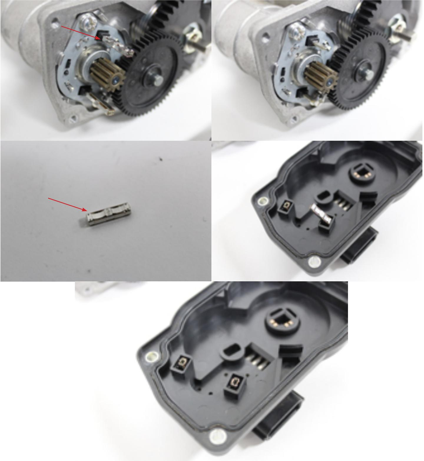
5. Remove the intermediate gear. Set it to the side.
