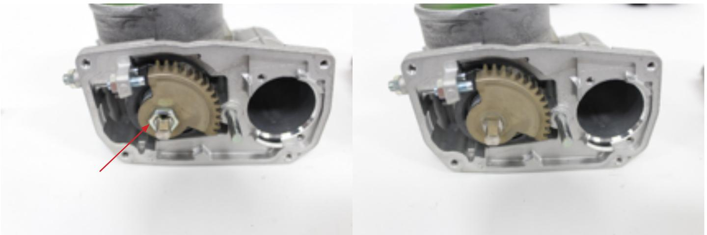
8. Remove the throttle shaft gear. Pay close attention when removing. This gear is under spring tension. Note how the tension is applied. Remove the spring underneath and set both to the side.
