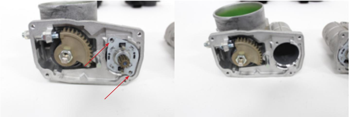
7. Remove the 12mm nut retaining the throttle shaft gear. Set to the side.
