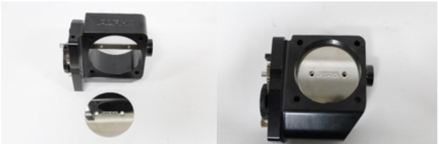
17. Apply red thread locker (Red Loctite) to the threads of the throttle plate screws. Install loosely.
