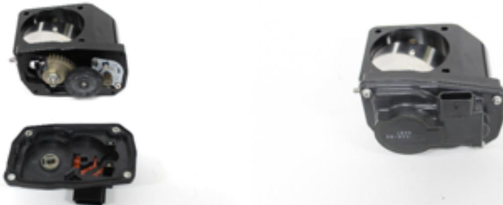
23. Install the Alpha endcap. Use green sleeve retaining compound on the mating edge of the endcap. Align and drive into place with a plastic or soft mallet.
