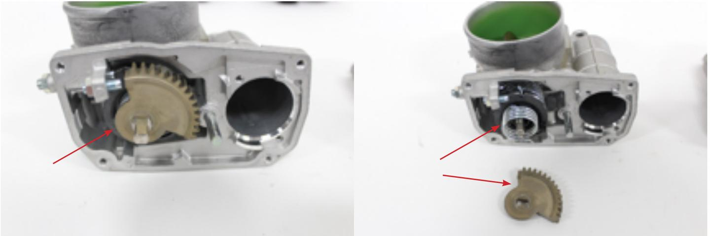
9. Remove the throttle stop cam. Pay close attention when removing. This stop cam is under spring tension. Note how the tension is applied. Remove the spring underneath and set both to the side.
