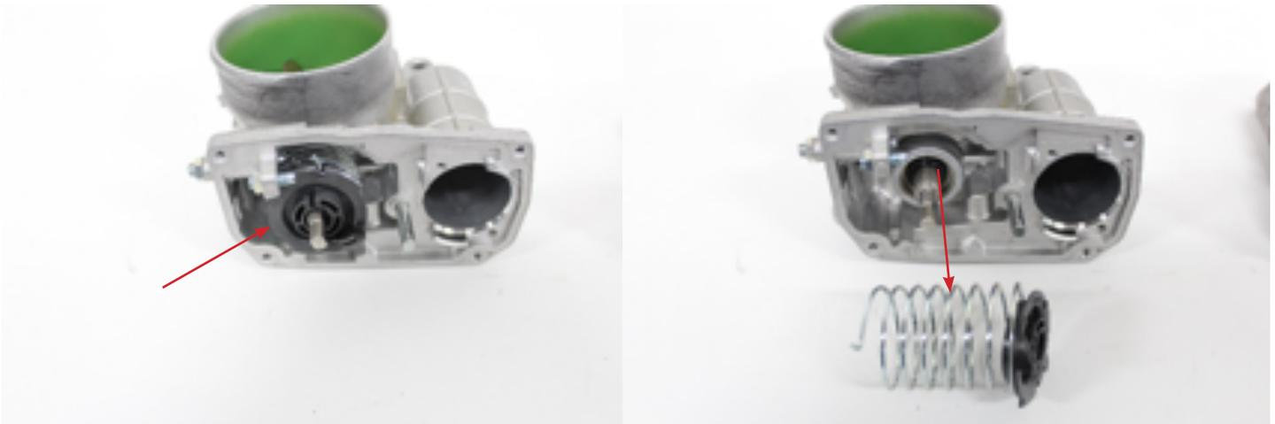
**Note: make sure the OEM components are only installed in the correct side they were removed, matching up the throttle body side to side. They cannot be swapped left for right.**
