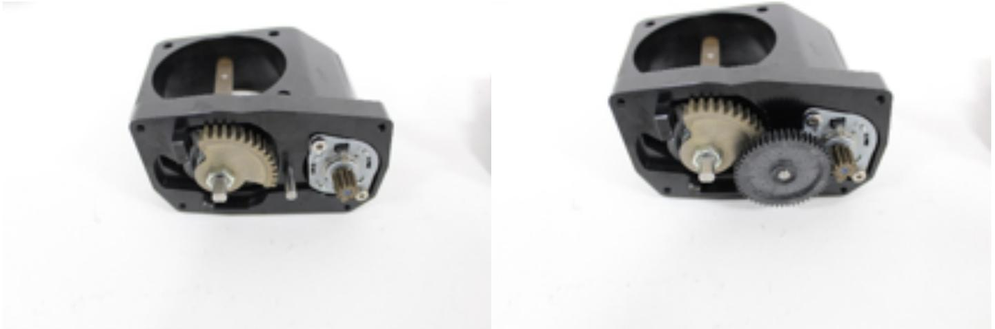
16. Insert the throttle plate into the throttle body housing. Make sure the throttle plate and housing are both facing a direction in which "ALPHA" can be read.
