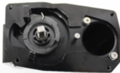
12. Check the rotational position of the throttle shaft. The “flat” of the shaft where the throttle plate secures to, must be facing outward. Outward can be determined by orienting the throttle body in a position that the “ALPHA” engraving on the top of the throttle body can be read.
