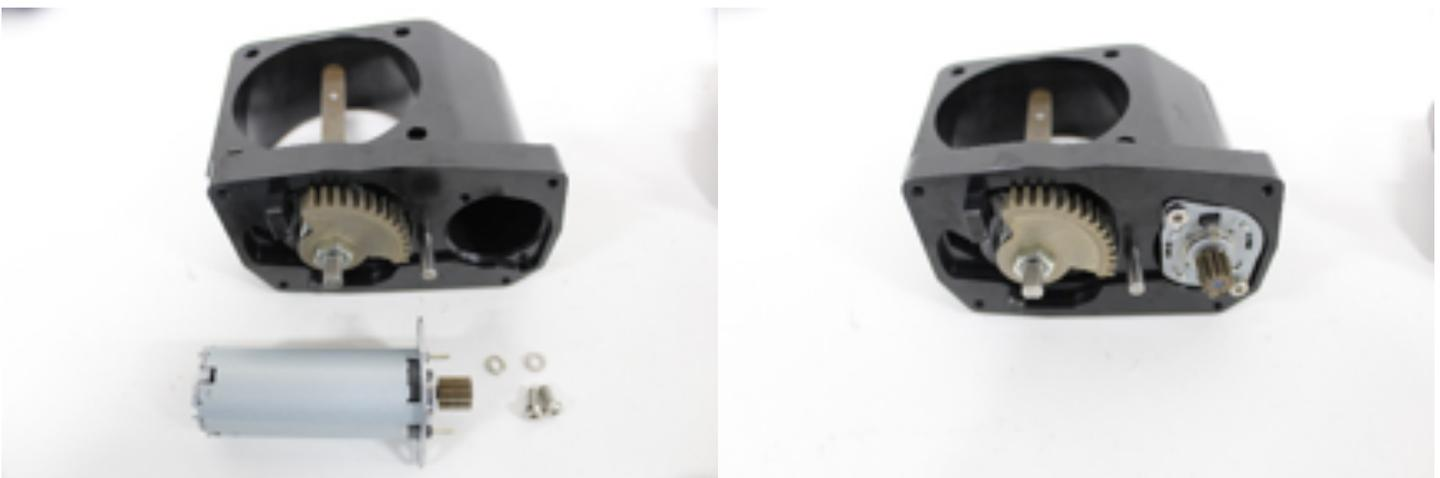
15. Install the intermediate gear.
