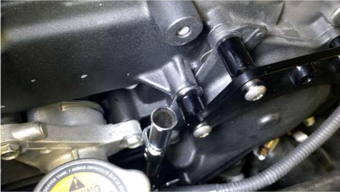
6. Re-install serpentine belt idler pulleys. And re-tension belt by removing lock bolt from tensioner. Be sure to check belt routing and position on the pulleys.
