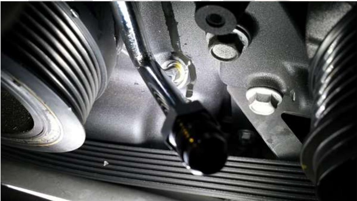
5. Remove 2 timing cover bolts as shown. Set aside. Attach Alpha air/oil separator bracket using 3 M6 stainless cap screws as shown. NOTE: one of the mount holes is shared with the dipstick tube.
