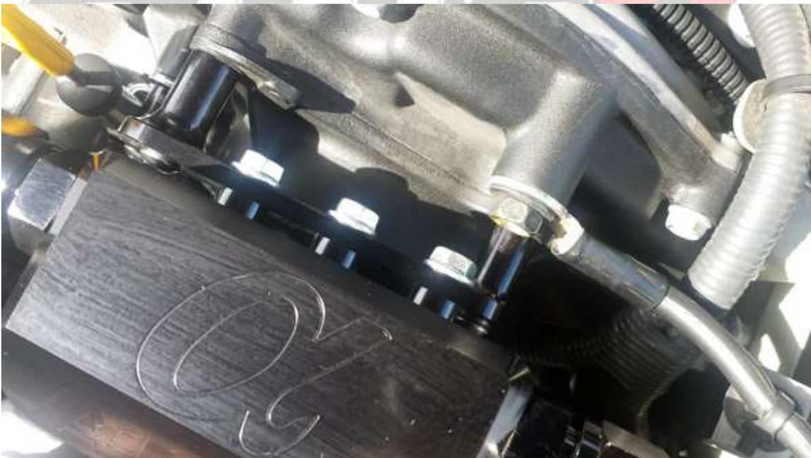
10. Check placement of -6 drain hose. Make sure it is free of any dangers/kinks. Final tighten fittings.
