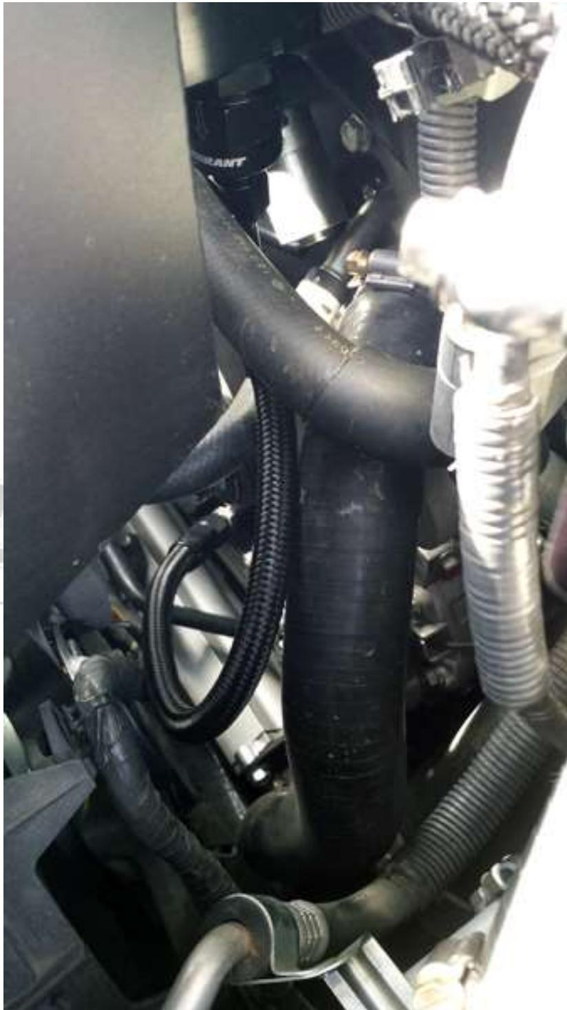
8. Set Alpha air/oil separator in place and attach drain hose (45deg fitting side) to bottom check-valve fitting. Leave loose.
