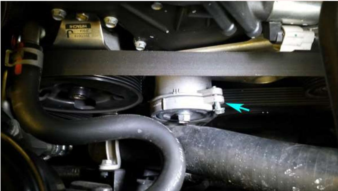
2. Use a 14mm socket/ratchet combo to remove 2 serpentine idler pulleys on engine.
