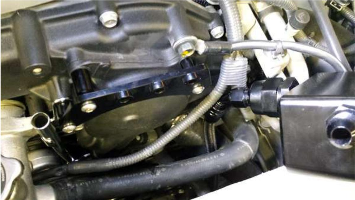
9. Maneuver separator into place on previously installed Alpha bracket. Attach separator to bracket using supplied M6 bolts(3), leave loose.
