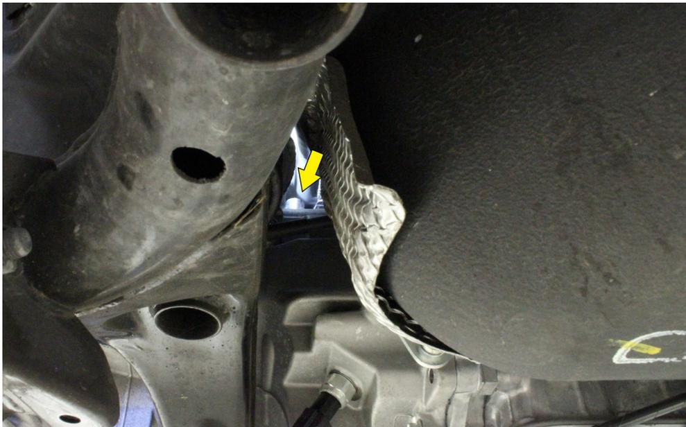
7. Install the hose and route the hose along the body above the transmission towards the fuel filler hose.
