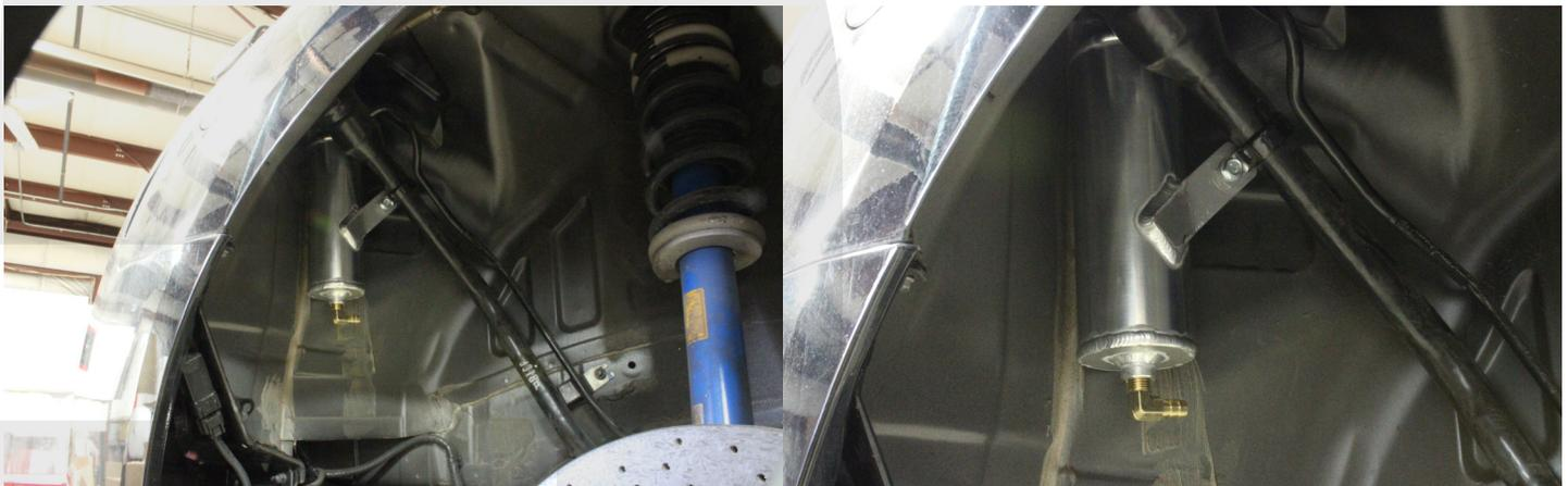
5. Locate the silver barb fitting on the top of the trans. Here is a picture of it with the transmission out of the car as well as where to find it in the car.
