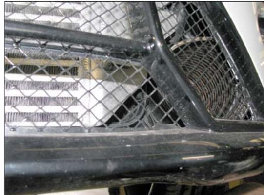
As the air pickup point is so low, common sense should be used when driving in very wet conditions – obviously do not try and cross any deep water likes fords or stream crossings, also be aware when following closely behind cars in the rain that extra muck and dirt will be pulled into the intake and reduce the service interval of the filter.
