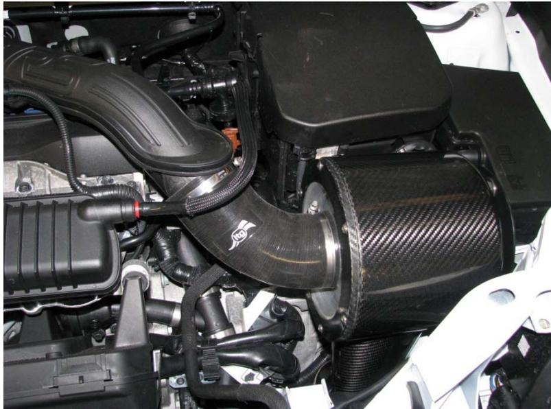
With the top part of the kit fully in place, you now need to tie down the cold air duct into place. There are plenty of places to wrap a cable tie round to be able to keep the ducting in place.
