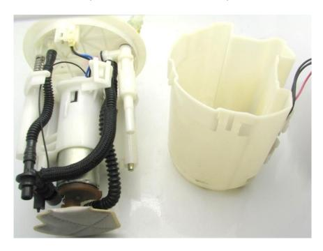
2 – separate the center section of the assembly from the top of the assembly by removing the C-clip (green) and disconnecting the venturi lines from the base of the center
