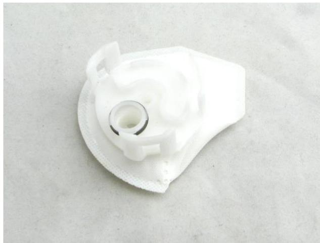
5 – transfer the outlet spacer from the OE pump to the DW pump and install 1 of the new orings from the installation kit. Install the new, clipped pre-filter on the DW65c/300c and install into the center assembly while connecting the electrical connector and snapping the pump retainer in place
