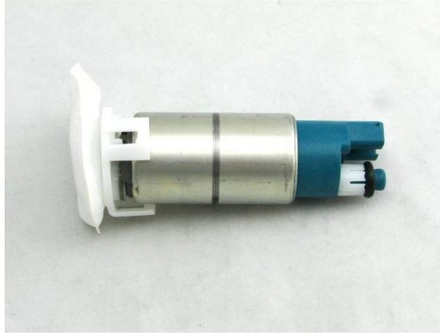
4 – prep the supplied pre-filter for use by separating the PRV retainer from the pre-filter. The PRV retainer will be discarded as the OE PRV retainer will stay on the center assembly
