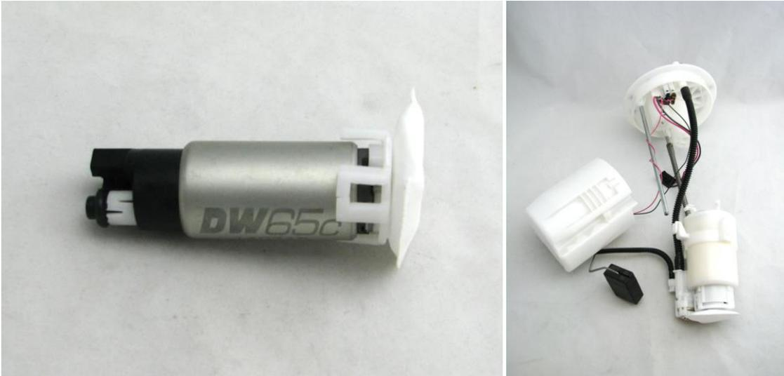
6 – install the assembly into the bucket and check to make sure all connectors are installed and wires are tucked in place, reinstall the vertical support retainers
