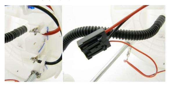
13 – reinstall the center section into the bucket, IT WILL NOT CLICK IN PLACE! Reinstall the top and c-clip and plug in the fuel pump connector and reinstall the fuel level sender and plug the connector into the top
