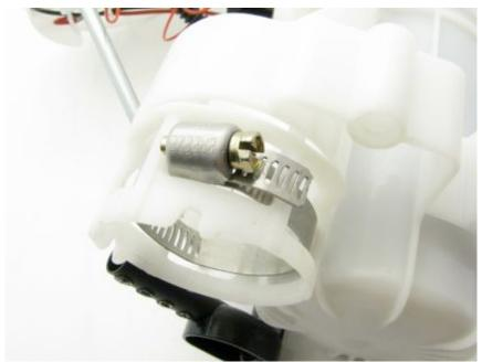
11 – install the DW65c and tighten the clamp. It only requires a minimum amount of torque
