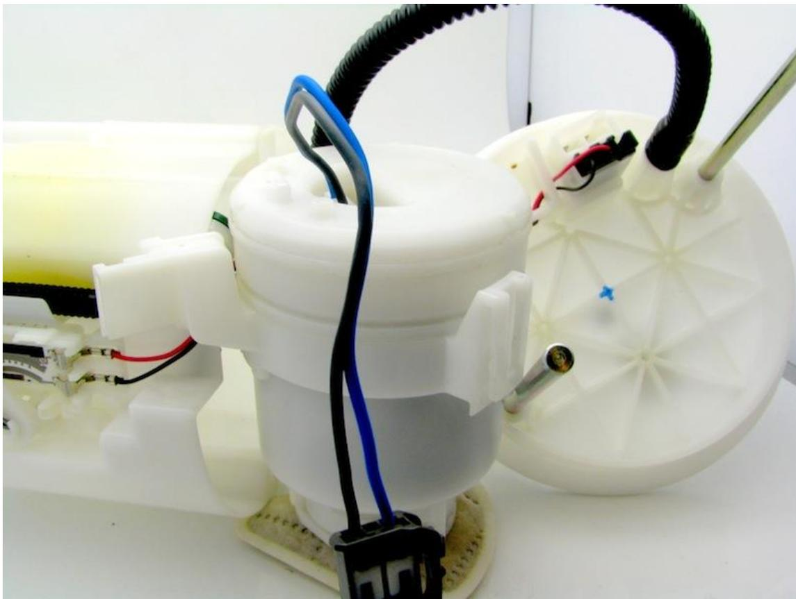
5 – five clips that hold the end cap for the fuel pump in the assembly
