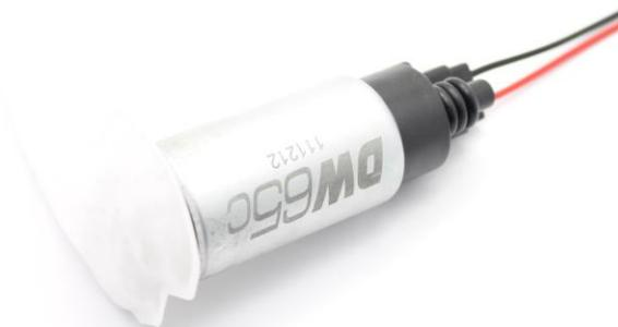
9 – install DW65c/300c into the center assembly and install into the bucket. Upon initial insertion, the pump may not be fully seated. If excessive effort is required to get the center section to clip into the bucket assembly, the pump is not fully seated into the center section, there may be a second “click” that occurs that indicates the pump is in place
