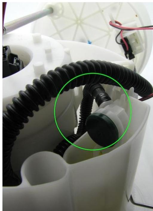
3 – three clips hold the bucket and the center together
