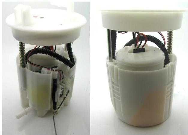
11 – reinstall the assembly into the fuel tank and attach a length of hose to the outlet of the pump assembly allowing it to drain into a fuel safe container and prime the fuel pump assembly
