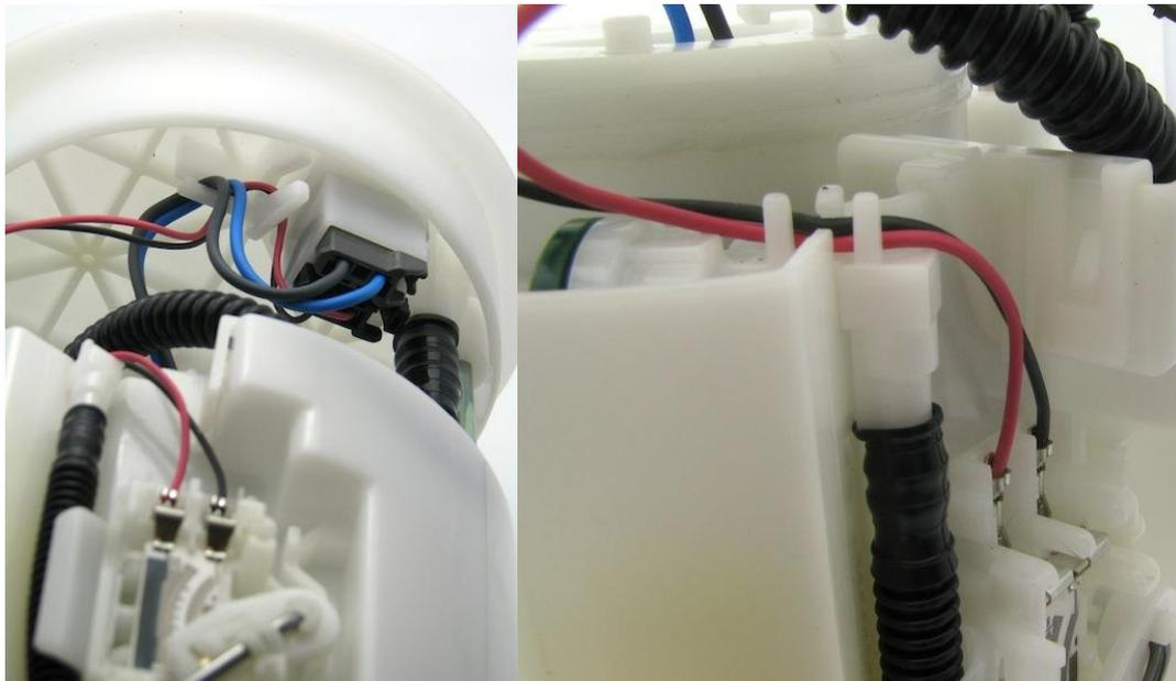
1 – remove retaining clip from vertical support
