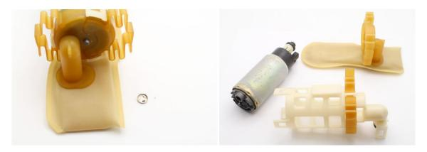
6 – transfer the oring spacer from the outlet of the OE pump to the outlet of the DW65c and install into the pump cage. BOTH ORINGS FROM THE DW INSTALL KIT WILL BE USED ON THE OUTLET OF THE DW65c
