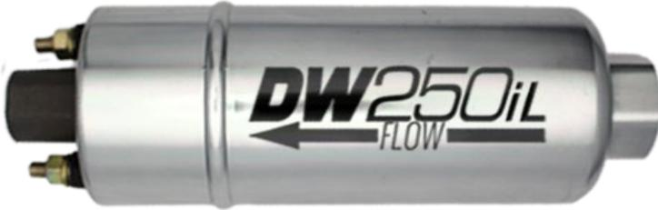
The DW250iL shares many of the same features as the popular DW350iL including: roller vane pumping mechanism, AN fittings, and anodized aluminum body. The DW250iL's small footprint, low current draw, and competitive price-point make it an ideal candidate for many builds targeting 400-600 HP. The 250iL is compatible with ethanol blended fuels but is NOT compatible with methanol or diesel fuels. All DW fuel pumps are backed by a 3-yr no-fault warranty.
