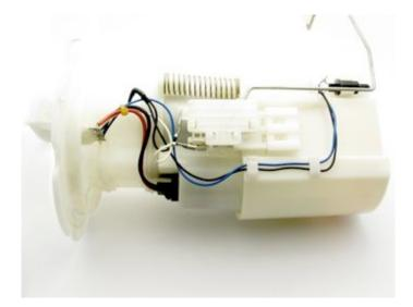
7 – reinstall the assembly into the fuel tank and attach a length of hose to the outlet of the pump assembly allowing it to drain into a fuel safe container and prime the fuel pump assembly
