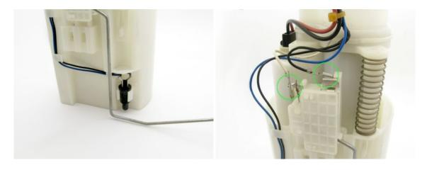
2 – lift the slide over the tab and pull the bucket away from the center section
