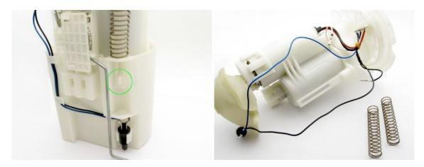
3 – pry the pump retainer off the center section and pull the pump out
