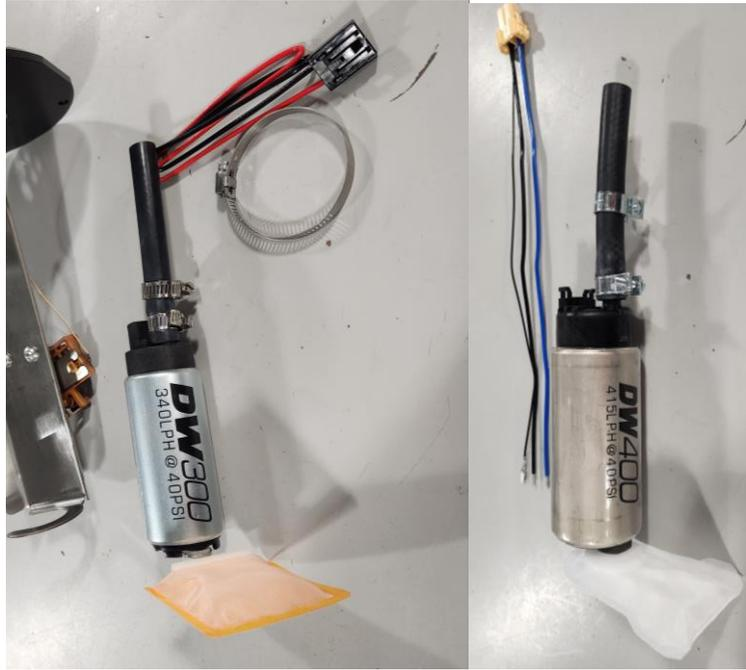
8 – Install the pumps into the hanger assembly, the filter sock will point the same direction as the fuel level float arm, this is important for fitment into the fuel tank. The pump is secured to the hanger assembly with the large 2-1/4" hose clamp, there are notches in the hanger to locate the clamp. Tighten the larger and small hose clamps.
