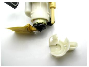
2 – unplug the stock fuel pump using a flat-head screw driver by pressing the tab in and twisting
