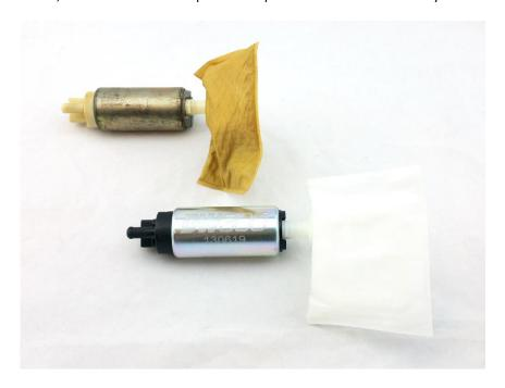
4 – measure and cut the supplied hose, then install it onto the assembly inlet. Slide the new hose clamps on the hose toward the top of the assembly and install the DW200/300 with the supplied isolator on the bottom of the pump. The supplied electrical connector is for earlier Impreza models that came with a different pump connector design. The OE connector can be retained
