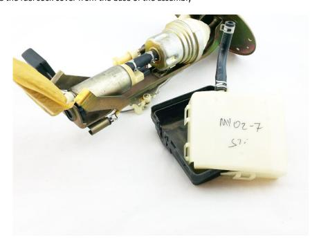
2 – loosen the hose clamps and push them up the hose toward the top, then pull the pump out of the assembly. Disconnect the electrical connector from the pump
