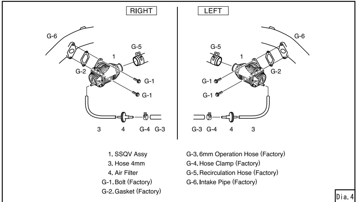
(2) Install the factory recirculation hose to both left and right SSQV Assy. (Dia.4)
