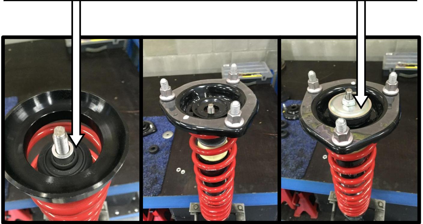
**Installing V-Maxx Autosport rear shockabsorber**
