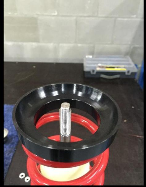
RE-use original strut bearing and install V-Maxx Autosport spring seat
