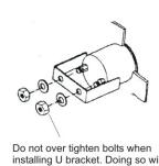
installing U bracket. Doing so will cause damage to movement inside.
