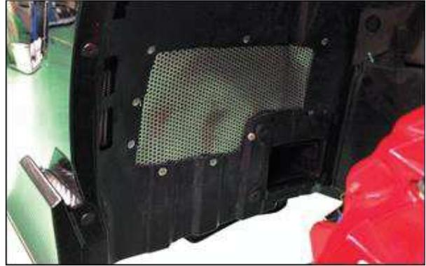
(15) Cut off the portion of ⑤ brake duct bracket LH along a dotted line as shown in the diagram.
