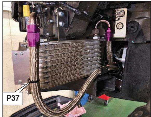
(27) Securely install the Oil Cooler Hose 1 to the Oil Cooler Core.
