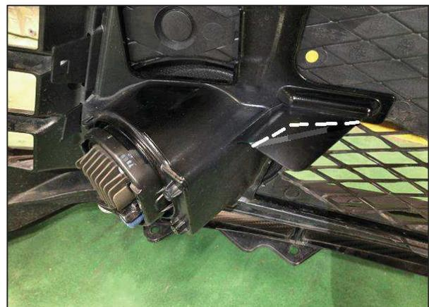
(18) Secure the wires shown in the diagrams below using the provided Tie Wrap S.
