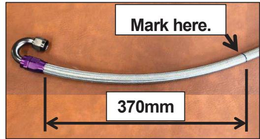
(25) Remove a protection cover from the 180° fitting attached to the Oil Cooler Hose 1 and 2. Temporarily install the hoses to the Oil Cooler Core.
