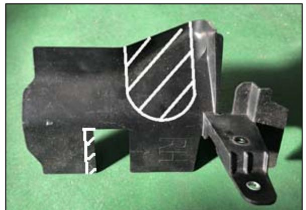
(24) Drill the  $\Phi 9\text{mm}$  hole(x2) to the Front bumper reinforcement.
