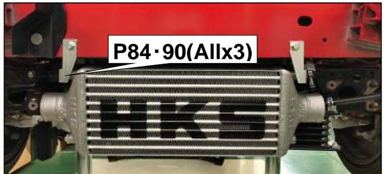
(8) Tighten all bolts of Intercooler and Intercooler bracket 1·2·3.
