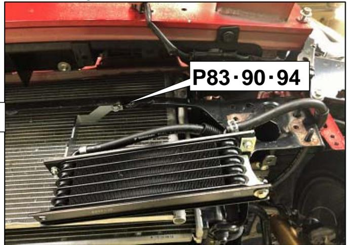
(19) Install the Hose  $\Phi 8$ (1) and (2) to the Supercharger & Traction fluid tank, and fix the hose  $\Phi 8$ (1) and (2).
