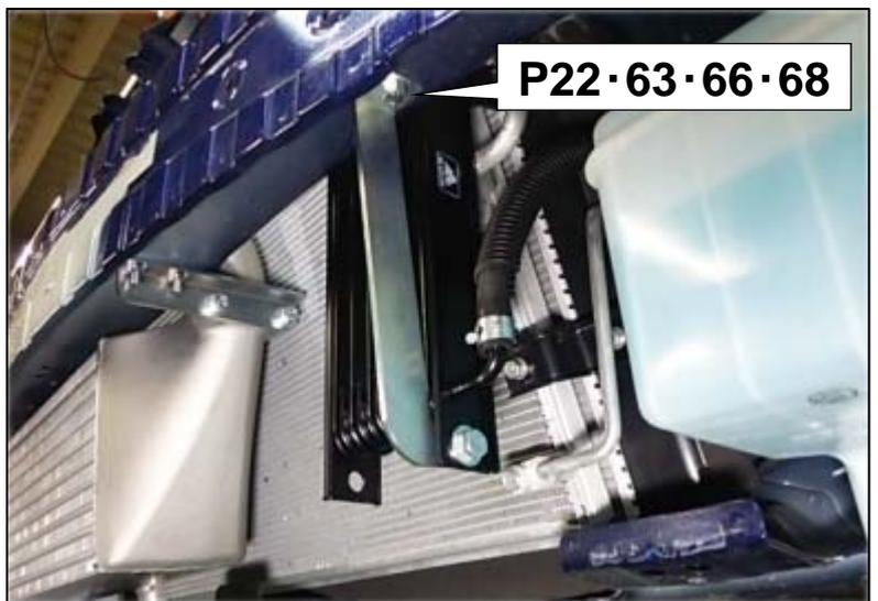
(14) Temporarily install the Traction Fluid Cooler Bracket No.1 to the front bumper reinforcement using the following provided parts.
