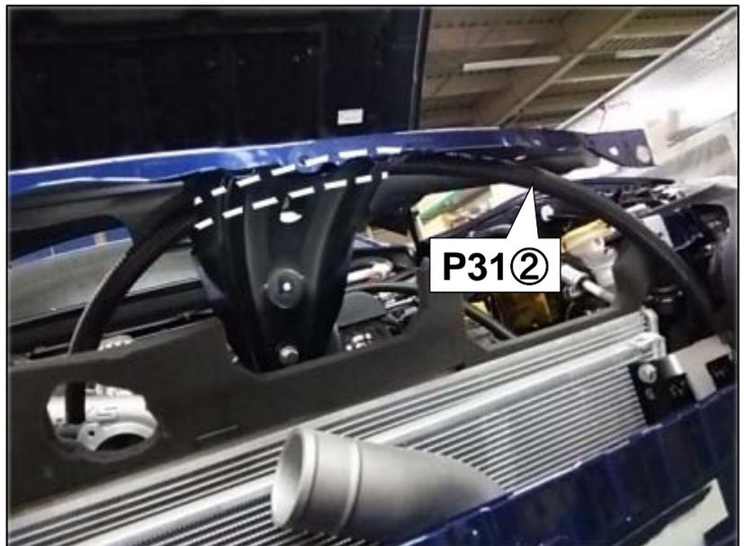
(18) Install the Traction Fluid Hose 8mm ② to the attachment on the upper side of the Traction Fluid Tank.
