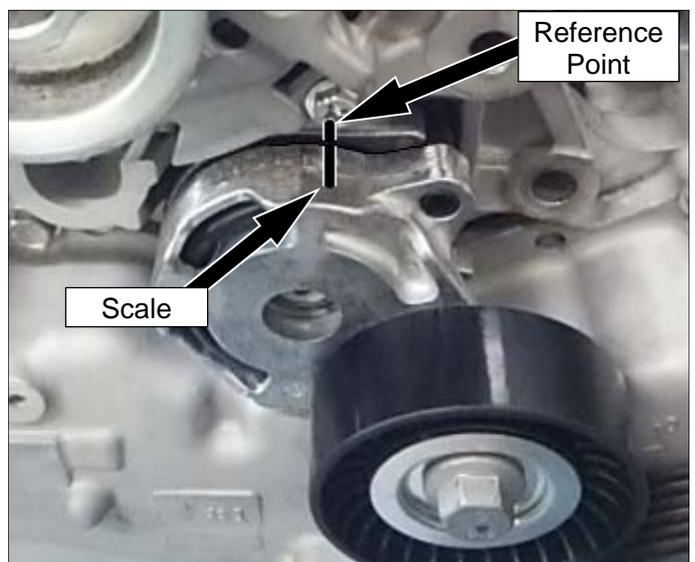
(23) Rotate Auto Tensioner pulley bolt to the right until it stops at the stopper. Mark another position where align with the reference point marked in (18).
