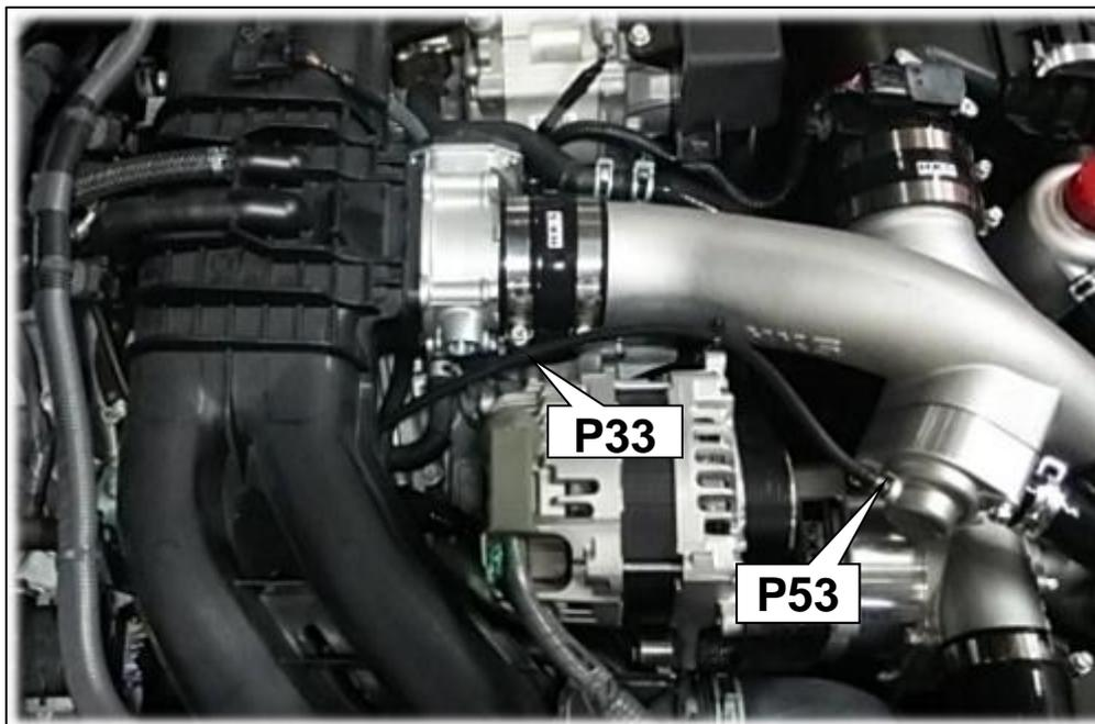
(13) Secure the Hose 4mm to the alternator using the provided Tie Wraps.
