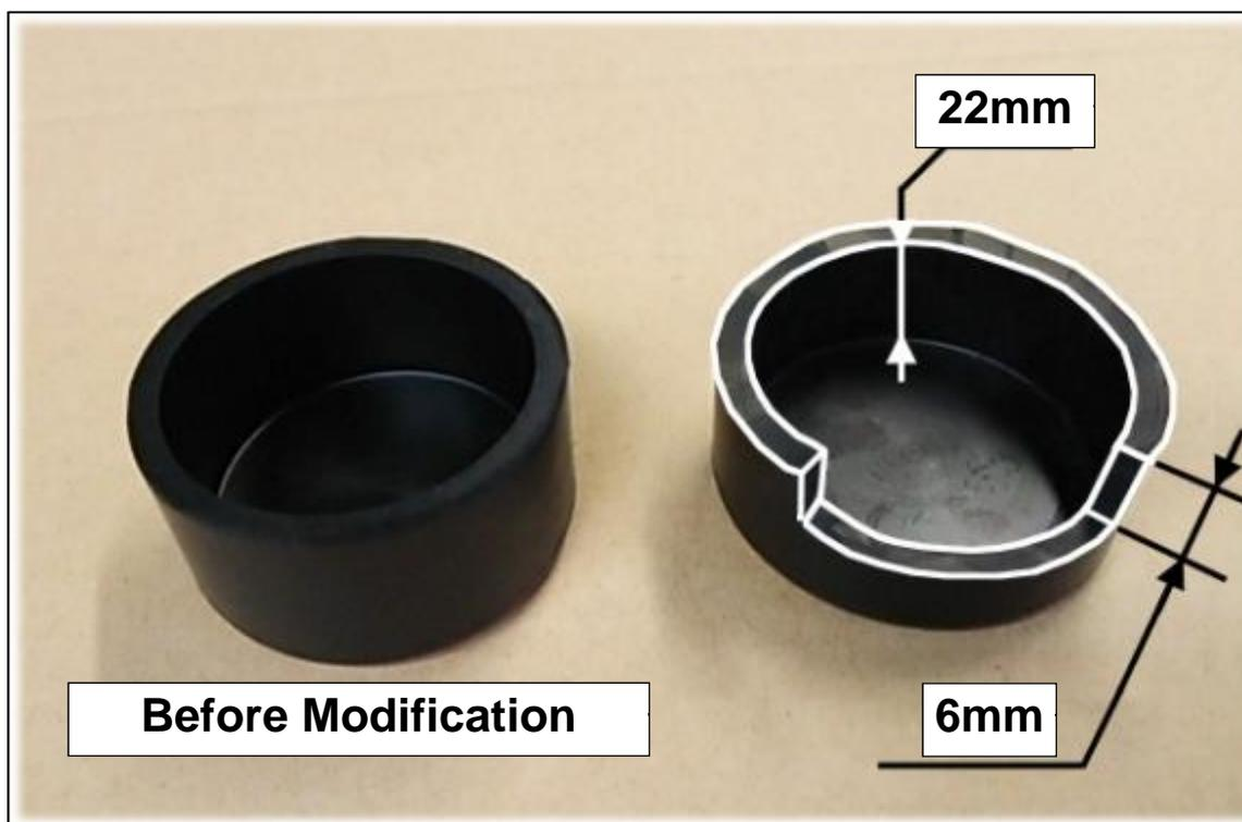
(33) Install the Rubber Cap 50mm modified in 2.(30) or 2.(32) to the position of the air cleaner where the resonator was removed in 2.(28).
