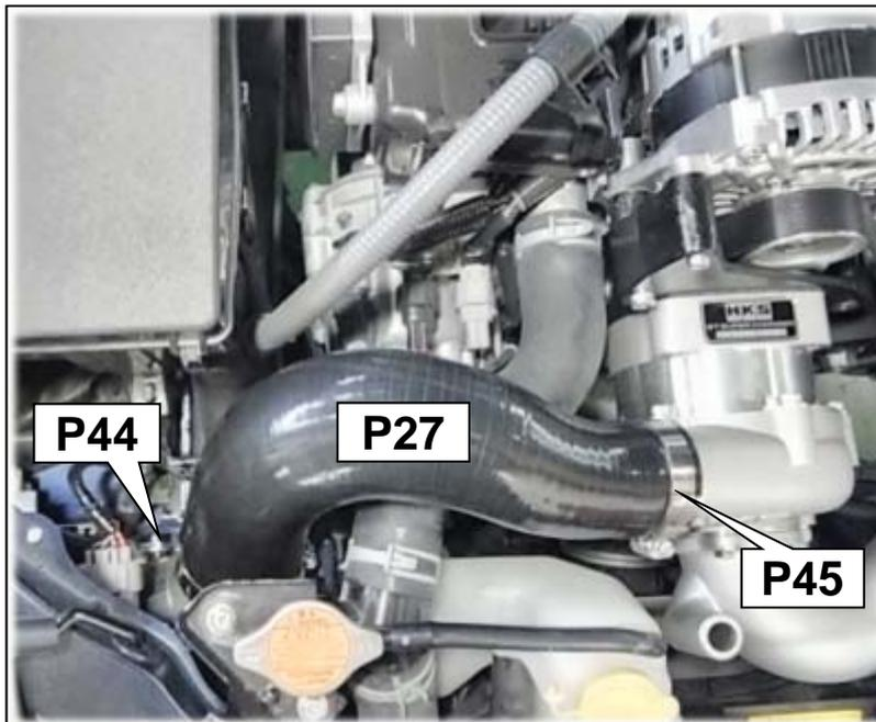
(8) Install the Intercooler Outlet Pipe No.1 and No.2 to the Intercooler and throttle.
