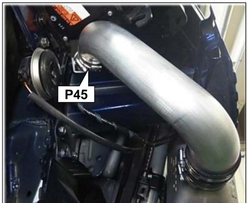
(7) Install the Silicone Hose 50mm-60mm to the GT2 Supercharger and Intercooler Inlet Pipe.
