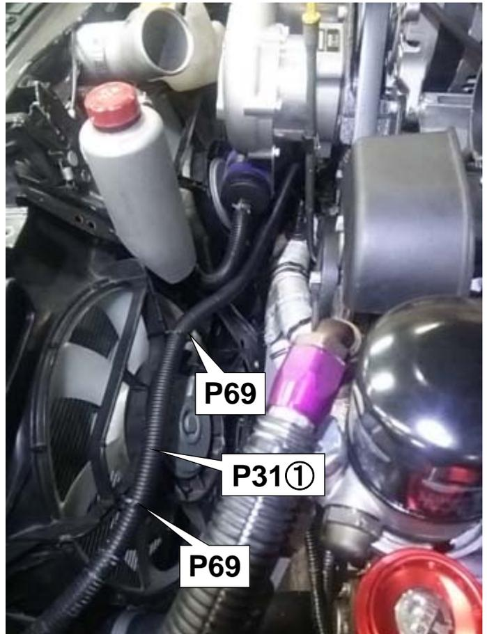
(23) Make sure there are no foreign objects in the Traction Fluid Tank. Add the Traction Fluid up to the dotted line in the diagram. Close the cap properly and securely.
