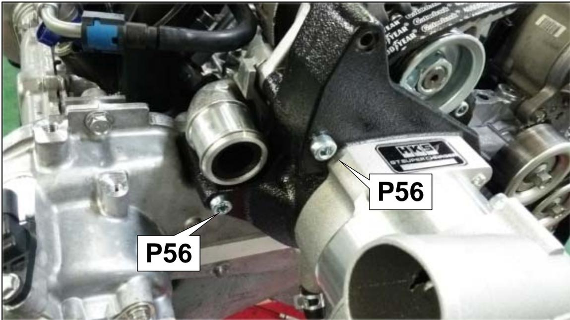
(6) Make sure the V-ribbed Belt is not caught in the Supercharger Bracket or engine. Tighten each cap bolt in several times in the order shown in the diagram below.
