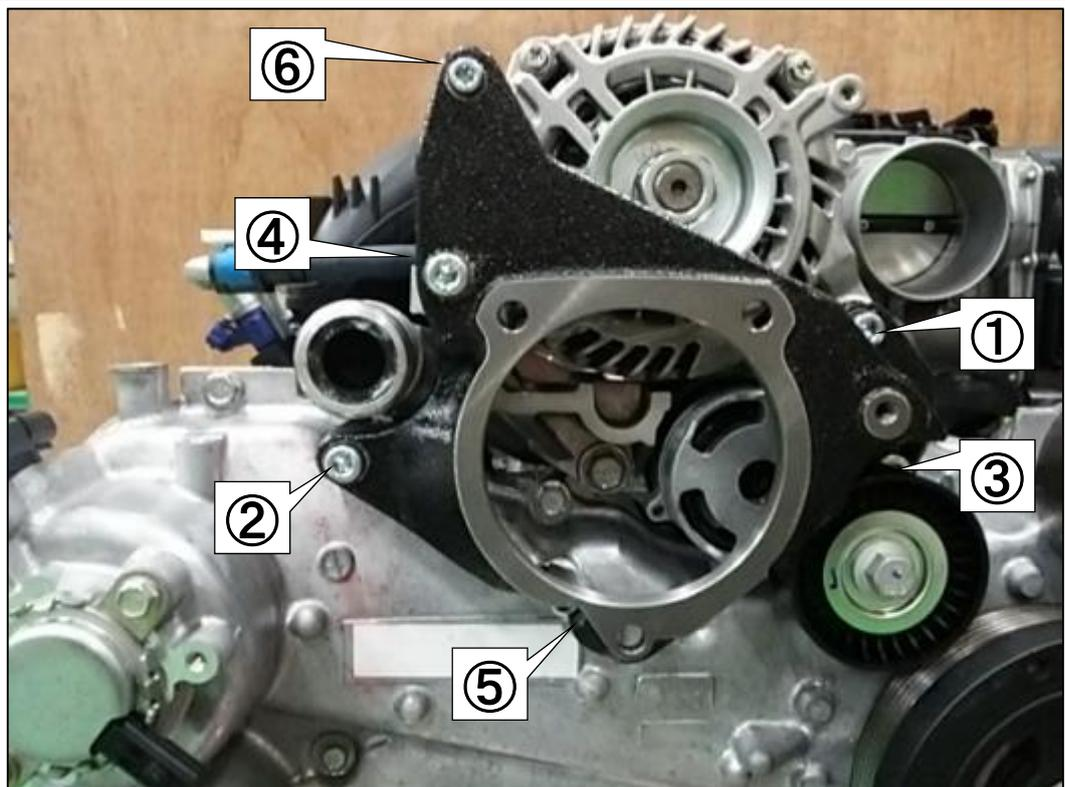
(7) Install the V-ribbed Belt temporarily installed in 3.(5) to \*7. Install the V-ribbed Belt to the engine.
