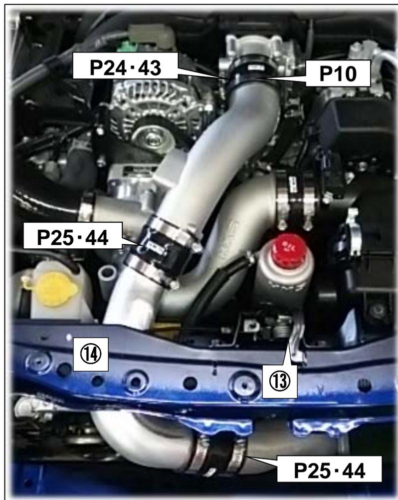
(9) Install ⑭ radiator support to the vehicle.
