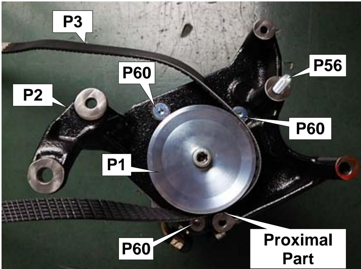
(2) Temporarily install the GT2 Supercharger to the Supercharger Bracket.
