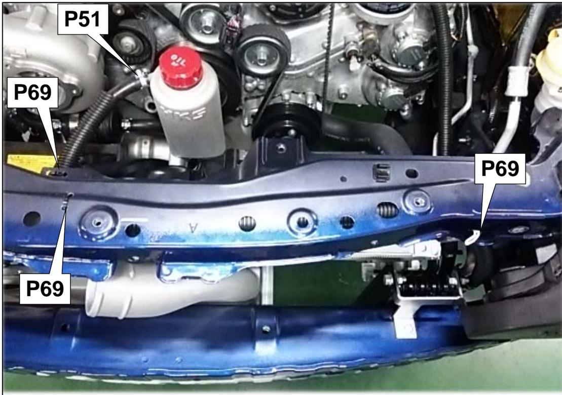
(19) Secure the Traction Fluid Hose 8mm ② to the Radiator Support in the position shown in the diagram above using the provided Tie Wraps (M). Pass the Tie Wraps through the holes made in 2.(13) and ones originally existed.
