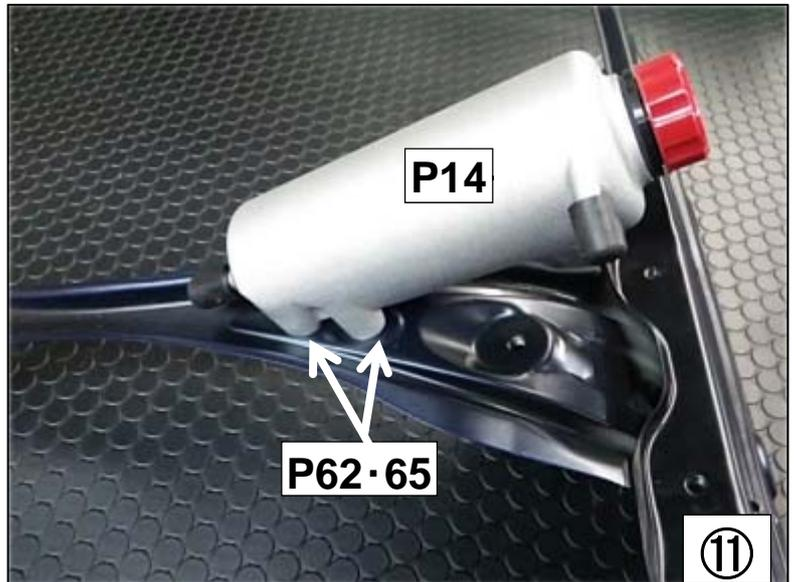
(17) Route the Traction Fluid Hose 8mm ② through the Radiator Support as shown in the diagram on the right. Temporarily install the Radiator Support to the vehicle.
