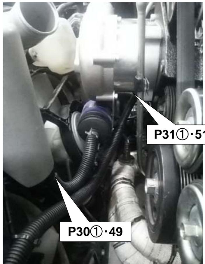
(22) Secure the Traction Fluid Hose 8mm ① to the radiator fan shroud using the provided Tie Wraps (M).
