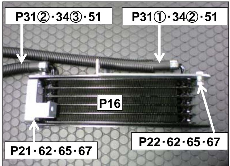
(13) Temporarily install the Traction Fluid Cooler Bracket No.2 to the front bumper reinforcement using the following provided parts.
