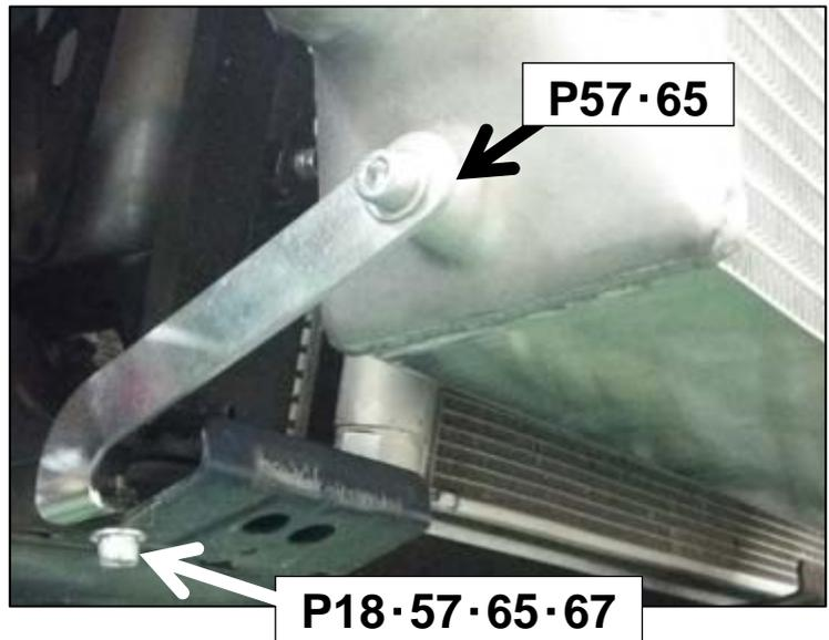
(3) Make sure the intercooler does not come in contact with any other parts of the vehicle. Tighten all bolts.
