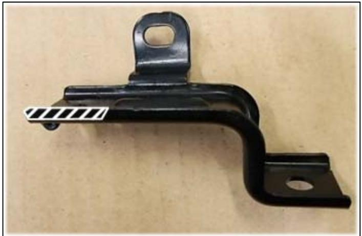
(2) Reinstall the A/C condenser bracket modified in 2.(1) to the original position.
