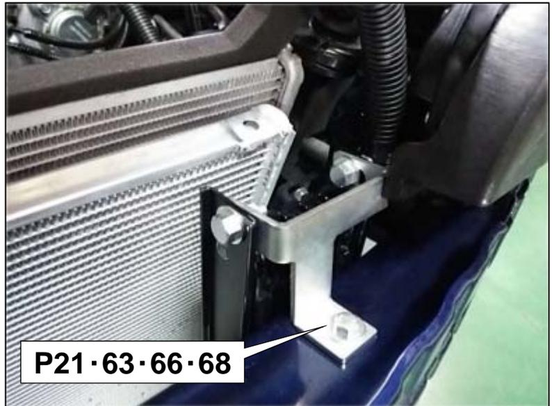
(16) Install the Traction Fluid Tank to the ① radiator support modified in 2.(12) using the following provided parts.
