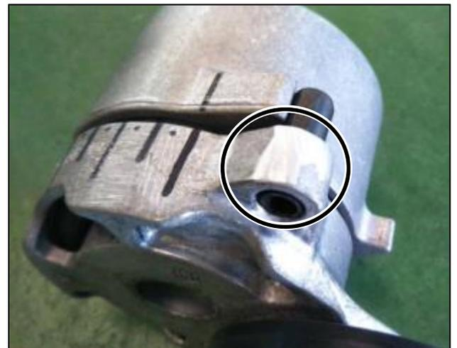
(22) For maintenance purpose, mark two positions on Auto Tensioner circled in the diagram on the right using an oil-based marking pen or a similar pen.
