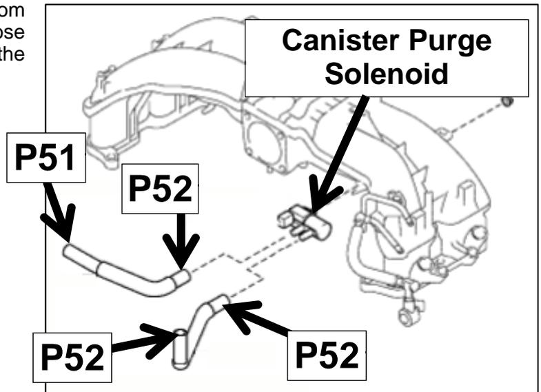
(40) Reinstall the canister purge solenoid. Place the throttle body and A/C compressor back in place.
