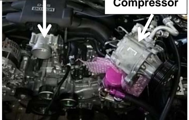
(38) Remove the installation bolt from the throttle body. Move the throttle body slightly so there is adequate space for installation function under the intake manifold.
