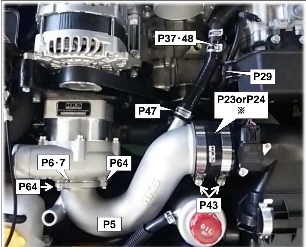
(3) Install the Silicone Hose 12mm-18mm to the Suction Pipe and Blow-by Hose.
