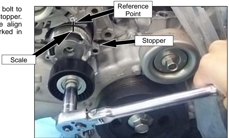
(24) Remove Auto Tensioner from the alternator bracket.
