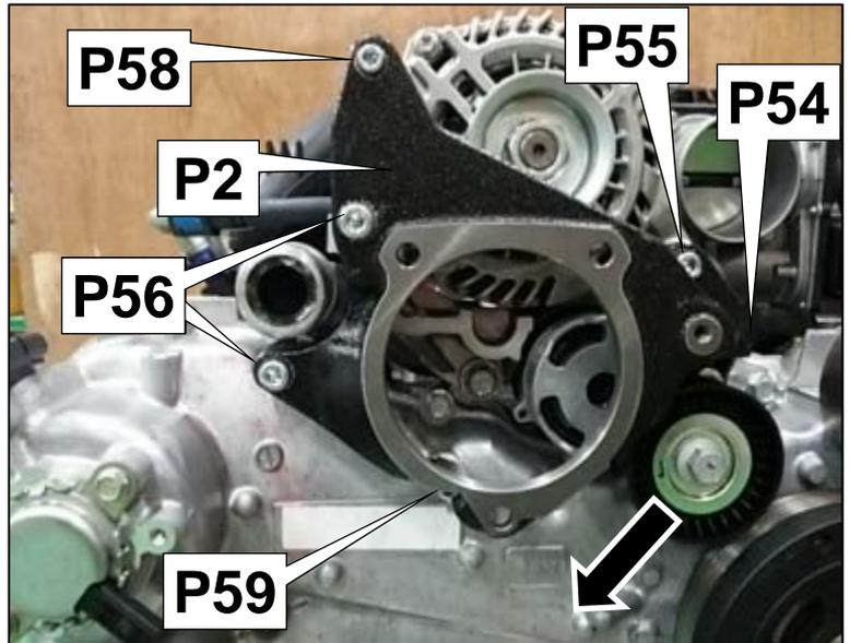
(20) Remove the Supercharger Bracket from the engine.
