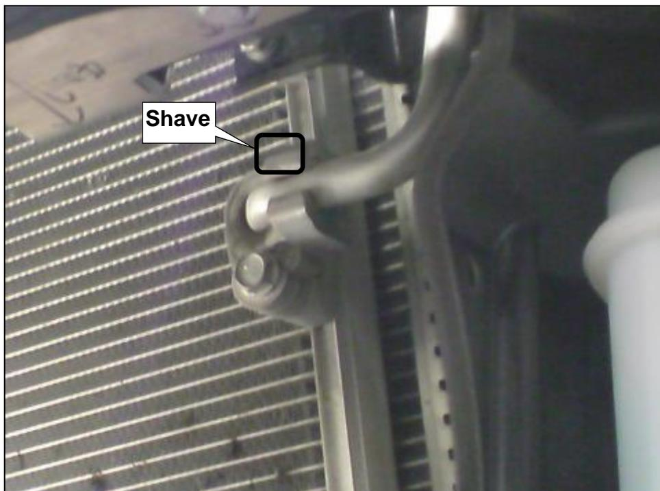
(6) Remove the bracket from ⑥horn removed in 1.(8).
