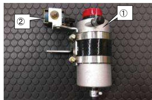
(10) Cut the Traction Hose Assy 10mm to ① 130mm and ② 900mm. Install these hoses to the Traction Oil Filter.
