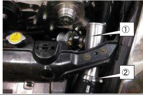
(8) Connect ②Hose 6mm installed in (3) to ①Blow-off Valve.
