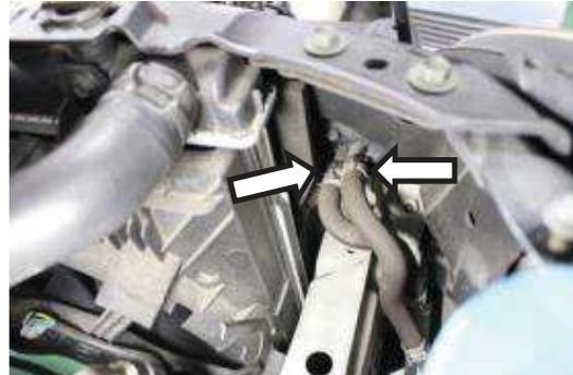
(19) Cut the provided Traction Hose Assy 10mm (②) to 2 of 240mm hoses. Install the provided Hose Clamp 10mm (①) and Joint Pipe 10mm (③) to each hose.
