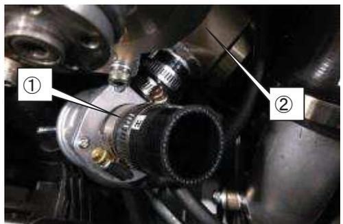
(7) install ①I/C Outlet Pipe No.1 and the Blow-off Valve temporarily installed in (6).
