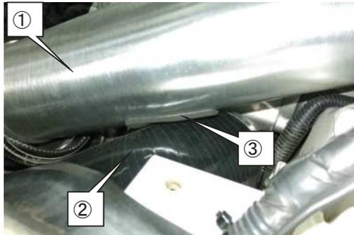
(11) Install ①I/C Outlet Pipe No.2. Make sure to install the airflow sensor coupler "A".
