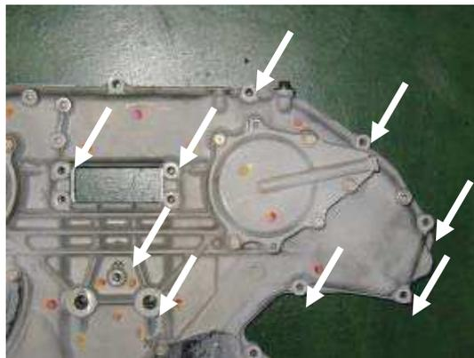
(5) Install the Supercharger Bracket No. 1 to the engine. To install the bracket, tighten ① bolt together with Bracket No.6, and ④ bolt together with the Bracket No.7.
