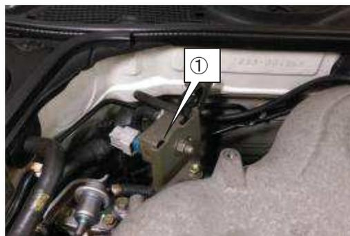
(8) Install ② Oil Tank Bracket to ① Traction Oil Tank using the following provided parts.
