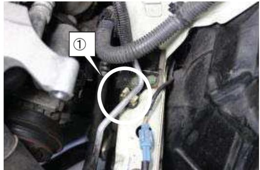
(11) Bend ①A/C pipe removed from the clamp in (10) in the direction indicated by arrows shown in the diagram. Wrap the pipe with the provided Corrugated Tube.
