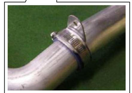
(11) Temporarily install the Intercooler Inlet Pipe No.1 assembly to the Supercharger Unit assembly.
