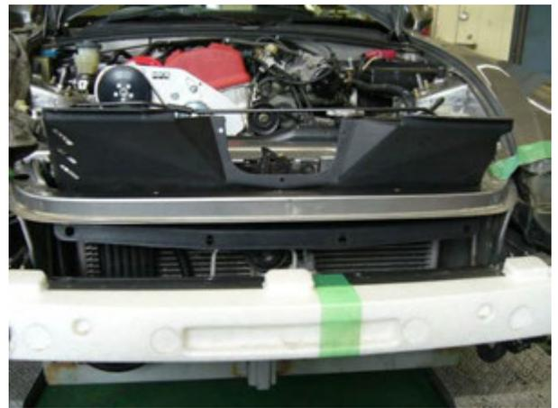
(18) Install the Traction Fluid Cooler Assembly to the vehicle using the following provided parts.
