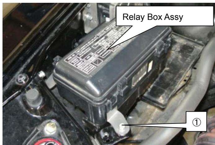
(24) Remove the clamp from the thick A/C pipe.
